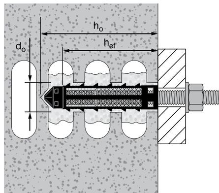
**Figure 6 - Hilti HIT-HY 70 specifications for Hilti HIT-IC in hollow masonry and brick with holes**
