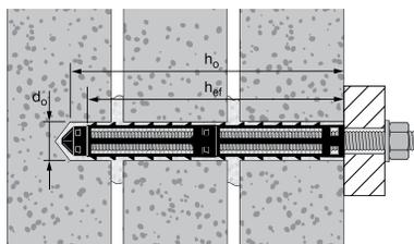
**Figure 8 - Hilti HIT-HY 70 specifications for rebar in multi-wythe brick wall**
