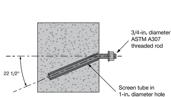
**Table 14 - Hilti HIT-HY 70 allowable adhesive bond loads for threaded rods in hollow core concrete panels<sup>1,4,5,6,7</sup>**
