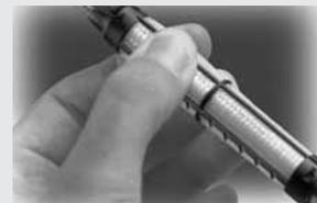
**Step 2:** Pierce the tip of the screen tube with the rod intended to be use to check embedment depth.
