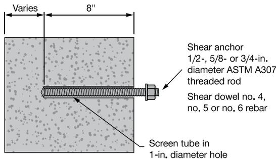
**Figure 10 - Hilti HIT-HY 70 with 22-1/2° combination anchor in configuration B**
