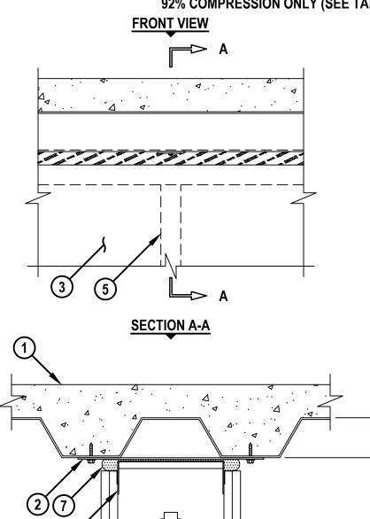
1. LIGHTWEIGHT OR NORMAL WEIGHT CONCRETE FLOOR (MINIMUM 2-1/2" THICK) OVER METAL DECKING ASSEMBLY (UL/cul classified). The Hourly fire rating of the Floor Assembly shall be equal to or greater than the Hourly rating of the Wall assembly.
