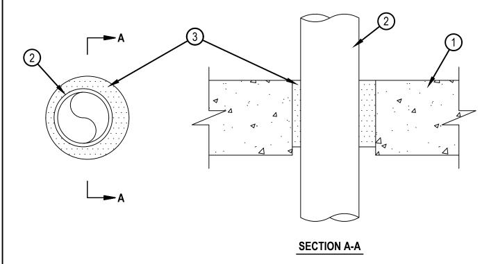
1. Floor or Wall Assembly — Min 4-1/2 in. (114 mm) thick reinforced lightweight or normal weight (100-150 pcf or 1600-2400 kg/m3) concrete. Wall may also be constructed of any UL Classified Concrete Blocks\*. Max diam of opening is 5 in. (127 mm).
