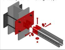
2. Base plate and through bolts - per analytical calculation
