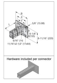
Hilti Hot-dipped galvanized bracket, typically used for fixation to a steel beam. The bracket is connected with beam clamps or using threaded rods through the slotted holes. Comes in different plate sizes to fit various steel beam sizes and in different lengths depending on application needs.
