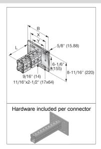
Hilti Hot-dipped galvanized bracket, typically used for fixation to a steel beam. The bracket is connected with beam clamps or using threaded rods through the slotted holes. Comes in different plate sizes to fit various steel beam sizes and in different lengths depending on application needs.
