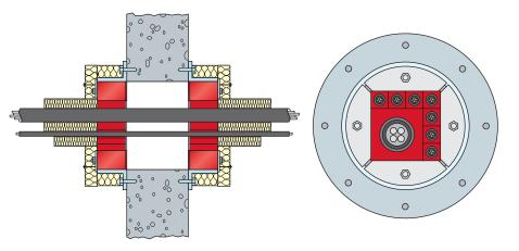
Rigid concrete floor with minimum thickness  $\geq$  200 mm.
