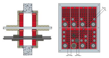
Rigid concrete floor with minimum thickness  $\geq$  200 mm.
