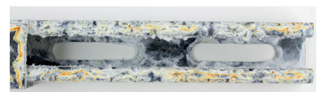
Fig. 31: Brown staining on a hot-dip galvanized channel after 200h in the salt spray test. No corrosion of the steel yet.
