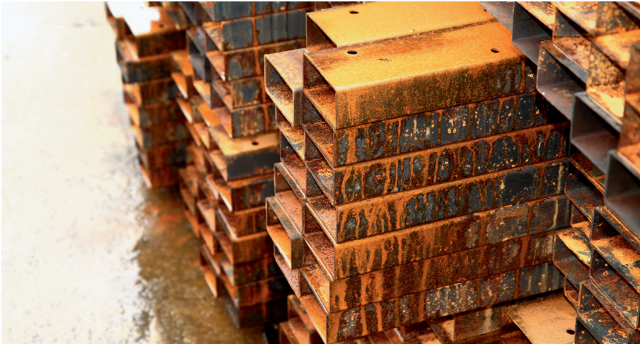
Fig. 4: Corrosion of steel components.
