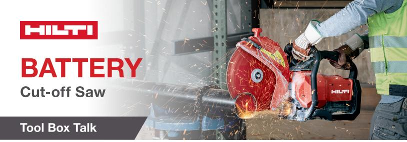
Second generation battery cut-off saws have built-in safety with kickback protection (active Torque Control-ATC) and better handling and maneuverability. Improper use of the tool can be dangerous. Below are some tips to keep in mind when using a battery cut-off saw:
