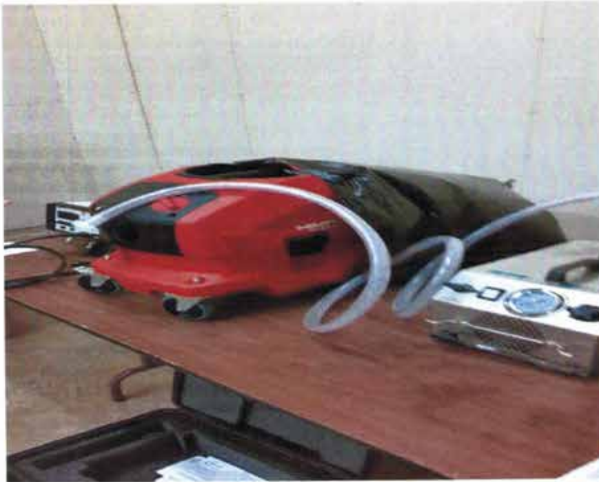
Test Setup showing Aerosol Generator on right HILTI VC20U Vacuum in middle with catch bag attached, and Aerosol Photometer on the left
