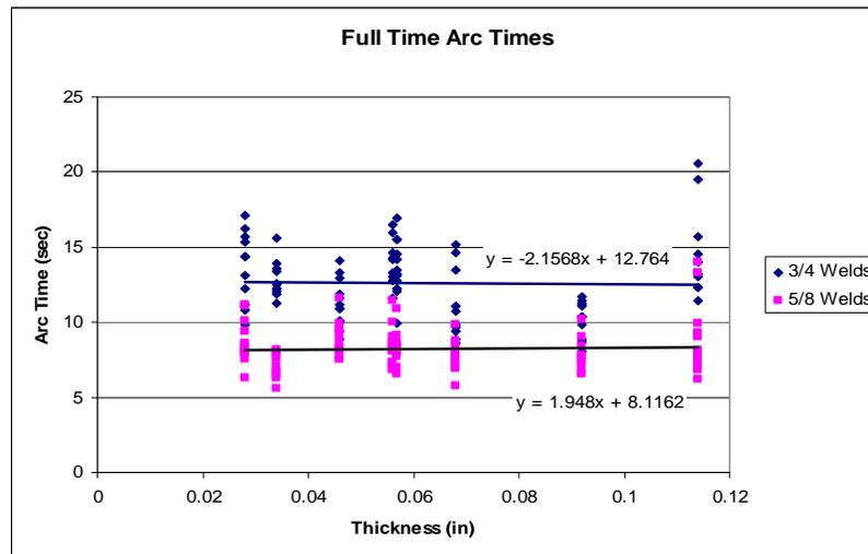
Figure 3-1: Arc Times for full-time Welds
