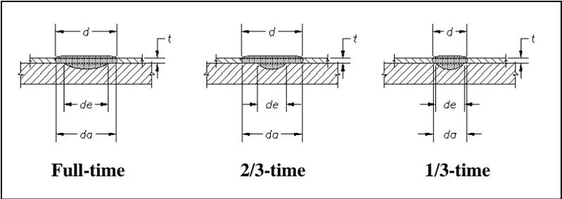
Figure 3-3: Common Weld Cross Sections
