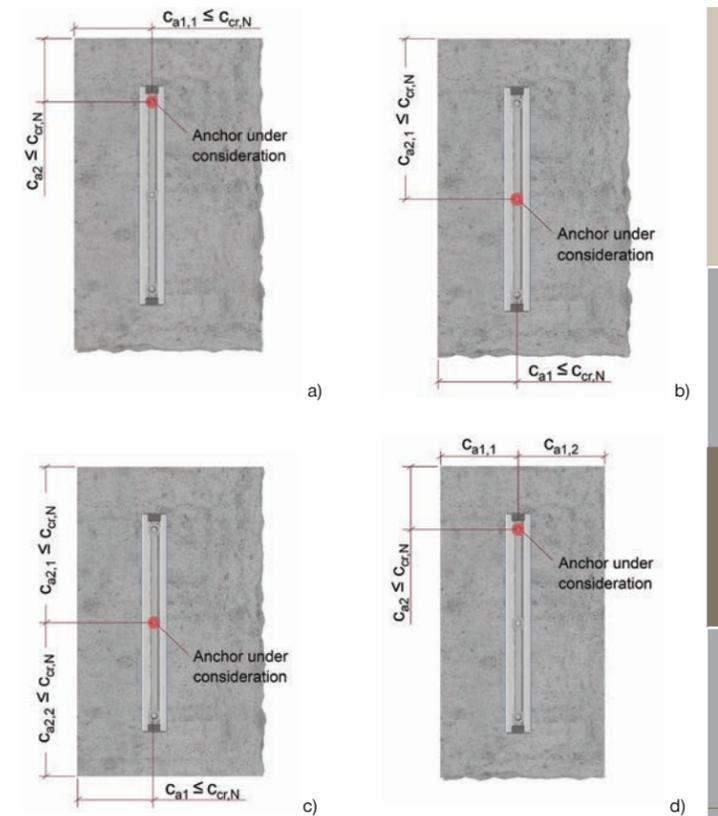
Figure 7.3.2.13 — Anchor channel with the influence of one edge and one corner (a and b), two corners and one edge (c), and two edges and one corner (d).
