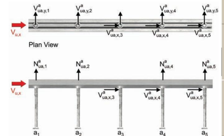
$$\begin{aligned} V_{ua,x,3}^a &= V_{ua,x,4}^a = V_{ua,x,5}^a = \frac{V_{u,x}}{3} \\ V_{ua,y,1}^a &= V_{ua,y,2}^a < V_{ua,y,4}^a = V_{ua,y,5}^a \\ N_{ua,1}^a &= N_{ua,2}^a < N_{ua,4}^a = N_{ua,5}^a \end{aligned}$$
