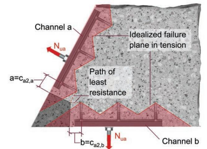
Figure 9.2.3.10 – Acute angle FoS corner with anchor channels on both sides – Tension analysis.
