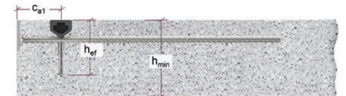
Edge distance ( $c_{a1}$ ) is measured from the face of the slab (outer face of the EDGE Plate).
