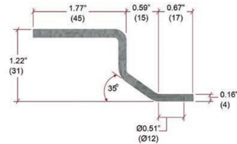
**Figure 2.2.16.10 — Geometry of S bracket, section view.**
