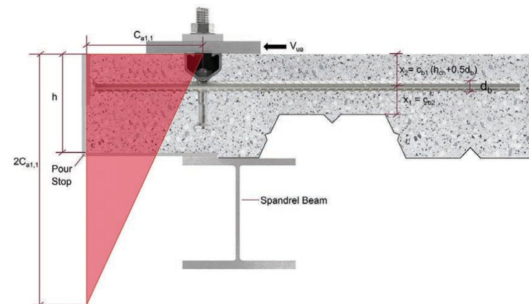
Figure 9.6.3.1 — HAC EDGE, HAC EDGE Lite and HAC S EDGE – Composite slab – Shear out.
