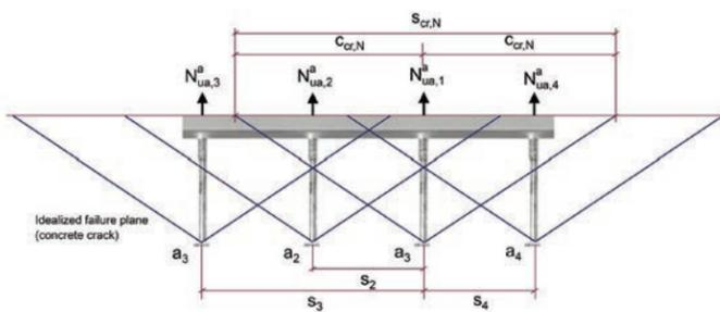
Figure 7.3.2.10— Example of anchor channel with non-uniform tension forces.
