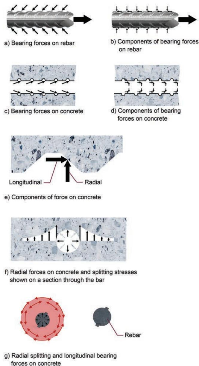
Figure 8.1.1.2 — Stresses and forces on a reinforcing bar and concrete. Source: Wight, James & MacGregor, James. *Reinforced Concrete Mechanics & Design*, 2012.
