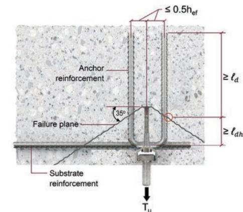
Figure 7.3.2.16 — Arrangement of anchor reinforcement for anchor channels loaded by tension load at an edge.
