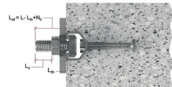
$N_h$  occurs after the installation torque is applied to the HBC-C-N t-bolt and the 2 mm deep notches are created in the lips of the anchor channel.
