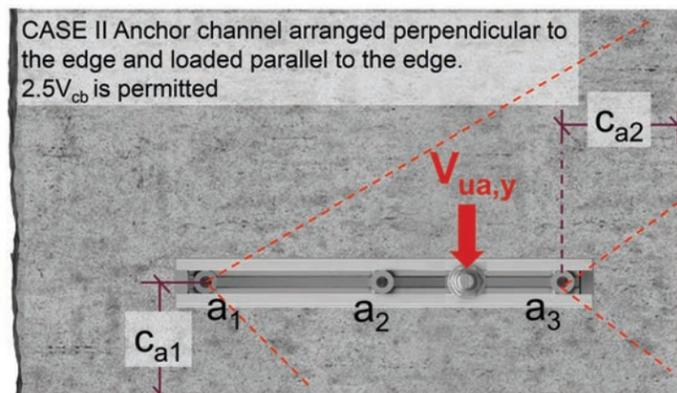
Figure 9.2.17— Anchor channel arranged perpendicular to the edge and loaded parallel to the edge.
