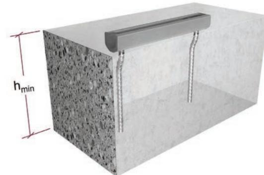
Figure 2.2.4.5 — Minimum HAC CRFoS U member thickness, isometric view.
