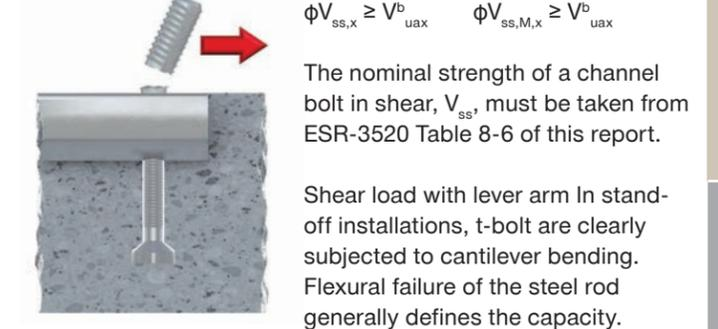
If the fixture is not clamped against the concrete but secured to the channel bolt at a distance from the concrete surface (e.g. by double nuts), the nominal strength of a channel bolt in shear,  $V_{ss,M}$ , shall be computed in accordance with Eq. (28).
