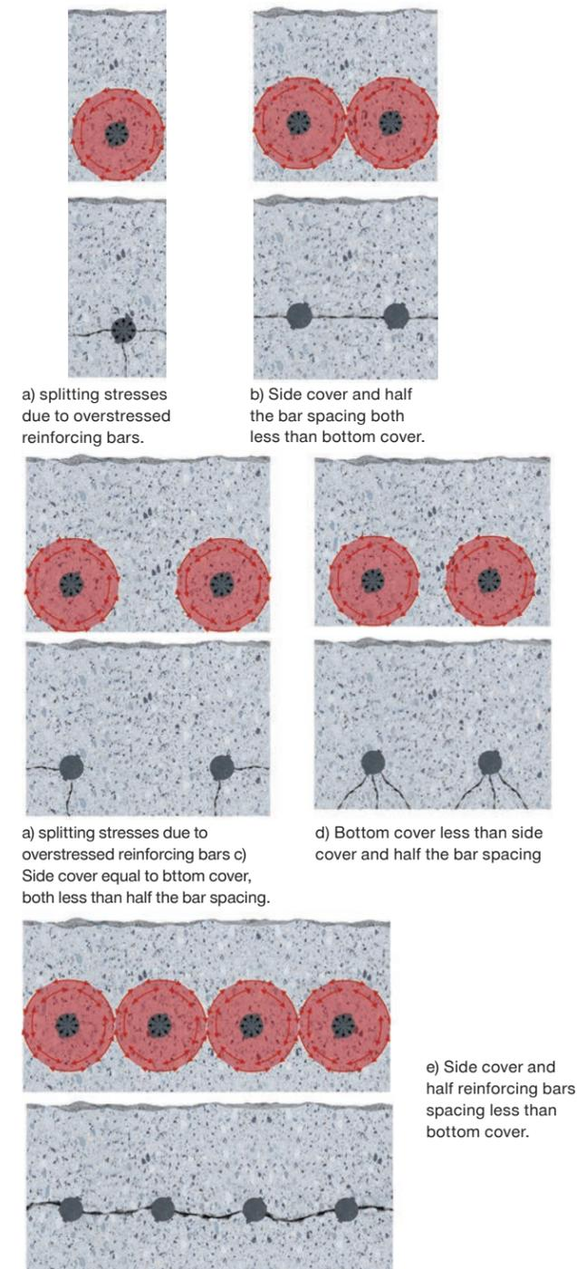
Figure 8.1.1.3 — Radial splitting stresses and splitting crack patterns. Source: Wight, James & MacGregor, James. *Reinforced Concrete Mechanics & Design*, 2012.
