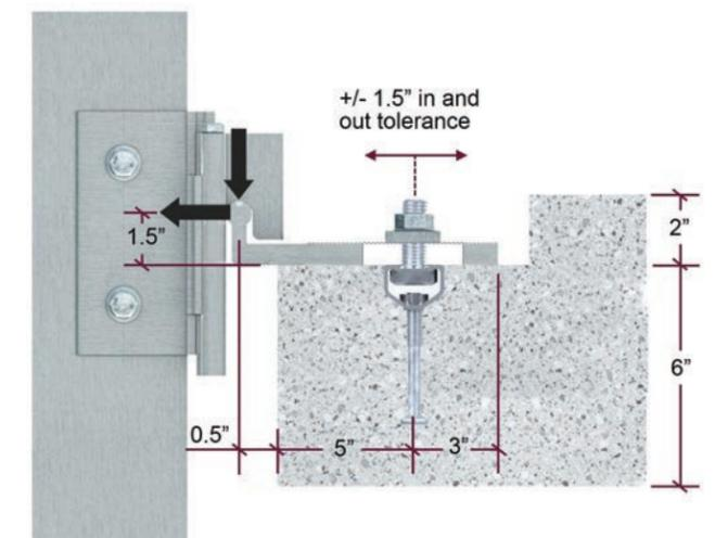
Figure 14.1.4 — Design example - Bracket Section View
