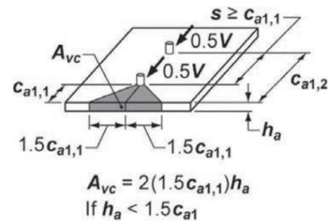
Figure 9.2.13.1— ACI-Fig. R17.5.2.1b—Calculation of  $A_{vc}$  for single anchors and groups of anchors per ACI 318-14..
