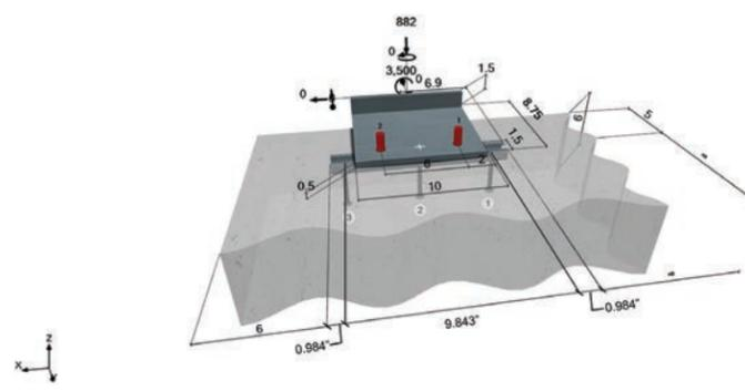
Figure 14.1.5— Design example – Profis anchor channel - 3D front View
