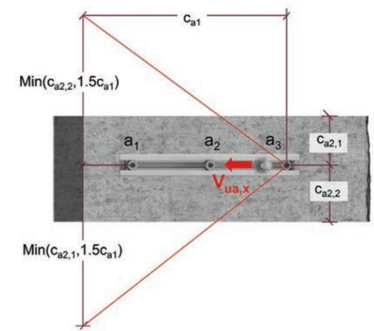
Figure 9.2.2.12 — Acute corner — Longitudinal shear — Plan view.
