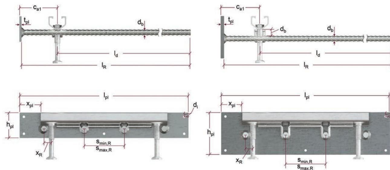
**Figure 2.2.16.8 — HAC-T EDGE Lite and HAC-T EDGE dimensions, section and elevation view.**
