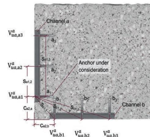
Figure 9.2.3.7.b – 90° FoS corner with anchor channels on both sides – Example of determination of  $\psi_{s,v,a1}$  – Section view.
