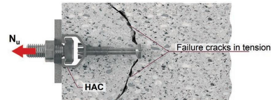
Figure 9.3.1.1 — Cast-in anchor channel with rounded stud anchors (HAC) loaded in tension.
