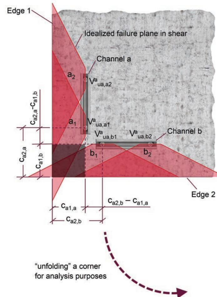
Figure 9.2.10.11c — anchor channels at the outside corner.
