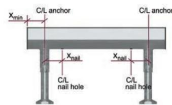
**Figure 2.2.16.5 b — HAC end and nail hole distance.**
