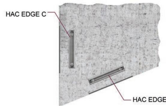
Figure 2.2.8.3 — HAC EDGE and HAC EDGE C in an acute corner, plan view.
