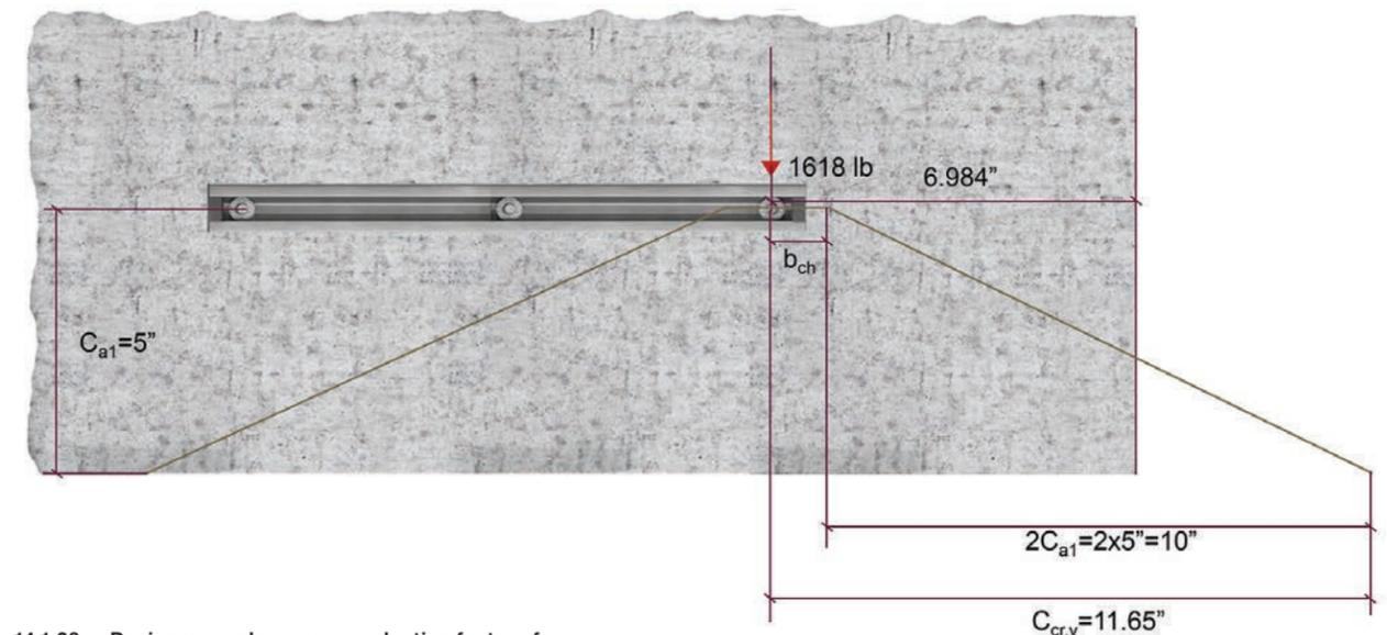
Figure 14.1.23 — Design example — corner reduction factor of  $\psi_{cr,v}$
