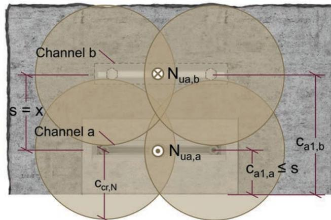
Figure 9.2.14.9 — Parallel Channels Top and Bottom-BOS away from TOS: Tension — TOS and BOS Plan View.
