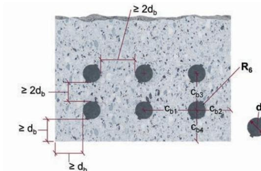
Figure 8.2.1.3 — Minimum reinforcing bar cover. Source: Wight, James & MacGregor, James. Reinforced Concrete Mechanics & Design, 2012.
