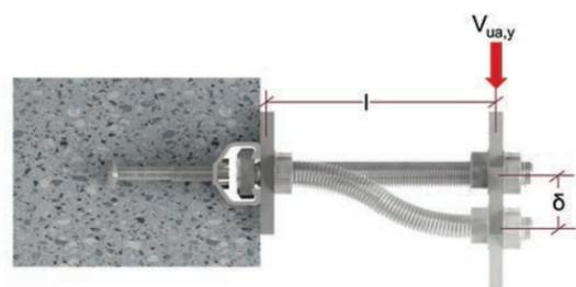
b)  $\alpha = 2$ ; fixture cannot rotate
