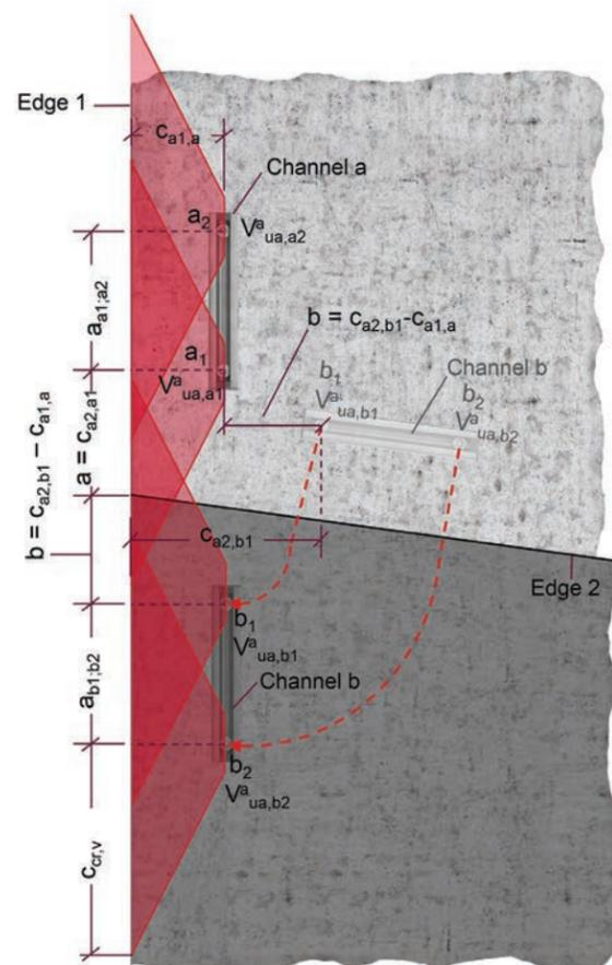
Figure 9.2.10.14b — Unfolding of Obtuse angle Corner.
