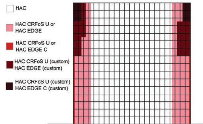
Figure 11.4.1.4 Anchor channel layout for conditions with extreme wind pressures
