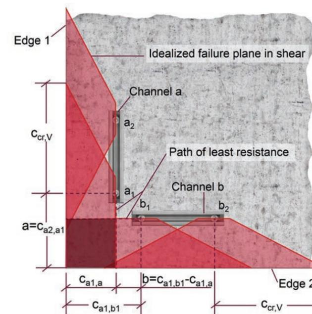
Figure 9.2.10.16-b— Simplified Method-90° Corner — Perpendicular Shear.
