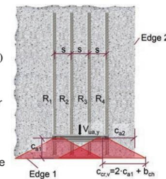
Figure 9.6.2.7 – Modification of corner effect:  $\Psi_{co,v}$
