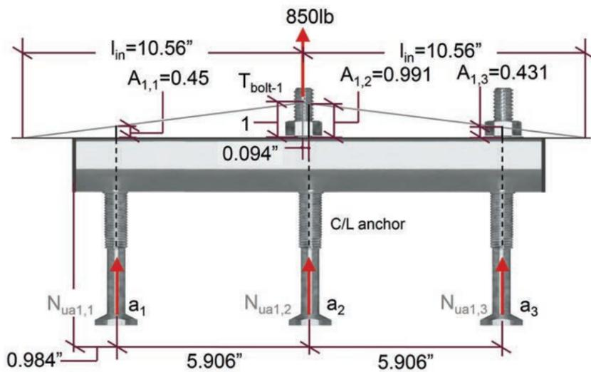
Figure 14.1.12 — Design example – effect of t-bolt 1 on anchors
