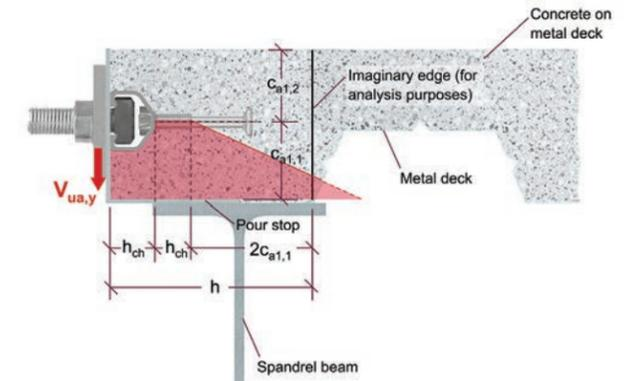
Figure 9.2.15.1-b — FOS: Composite Slab — Perpendicular Shear — Section View.
