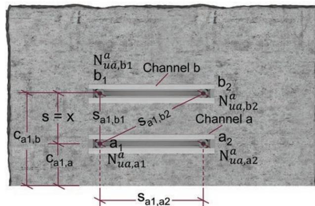
Figure 9.2.13.8 – Tension – unequal tension force-Section view.
