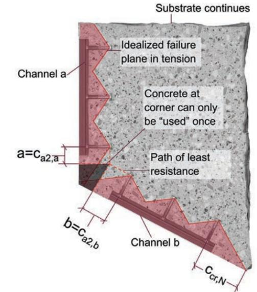
Figure 9.2.3.15 – Obtuse angle FoS corner with anchor channels on both sides – Tension analysis.
