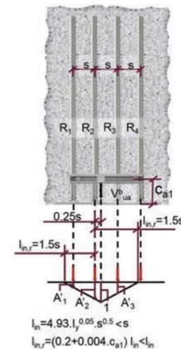
Figure 9.6.5.2 — Example for the calculation of rebar forces in accordance with the triangular load distribution method for an anchor channel with four rebars. The influence length is assumed as  $l_{in} = 1.5s$ .
