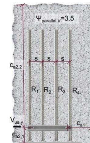
Figure 9.6.4.3 — TOS or BOS HAC EDGE single channel at certain distance — Shear along longitudinal axis x+.
