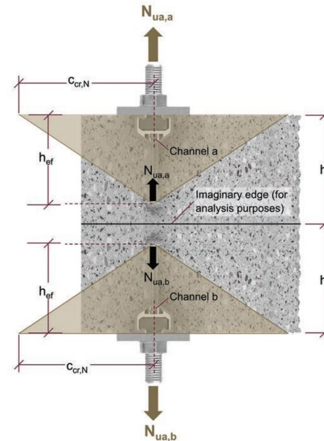
Figure 9.2.14.11 — Top and Bottom Channel: TOS under BOS -Tension — Section View.
