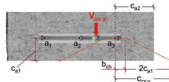
Figure 9.2.3.7.a – 90° FoS corner with anchor channels on both sides – Plan view.
