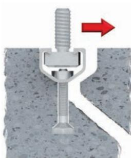
Concrete edge breakout failure: Failure of an anchor channel installed at the edge of a concrete member and loaded in shear towards the edge characterized by the formation of a fracture surface originating at the channel and projecting towards the edge of the concrete member as shown in the figure 7.4.2.1.
