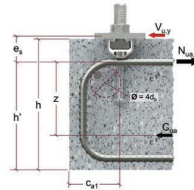
Figure 7.4.2.9b — Internal forces and detailing requirements for anchor reinforcement to resist shear loads; section view.
