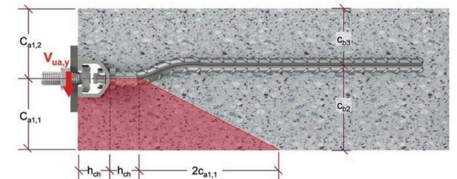
Figure 9.3.3.5 — HAC CRFOS U — Anchor channels on both sides — Acute angle Corner — Section View.
