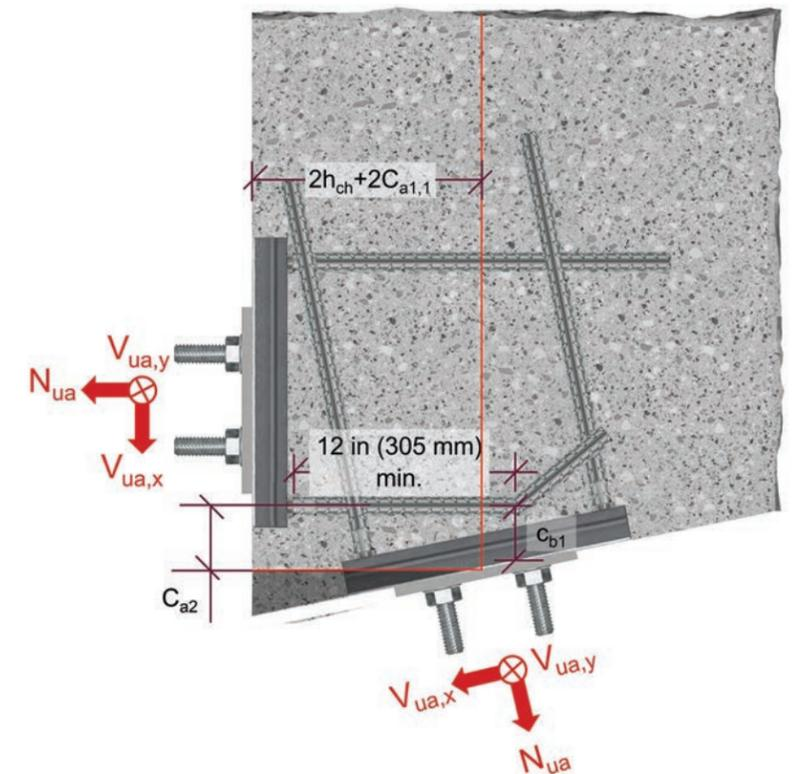
Figure 9.3.3.4 — HAC CRFOS U — Anchor channels on both sides — Acute angle Corner — Plan View.
