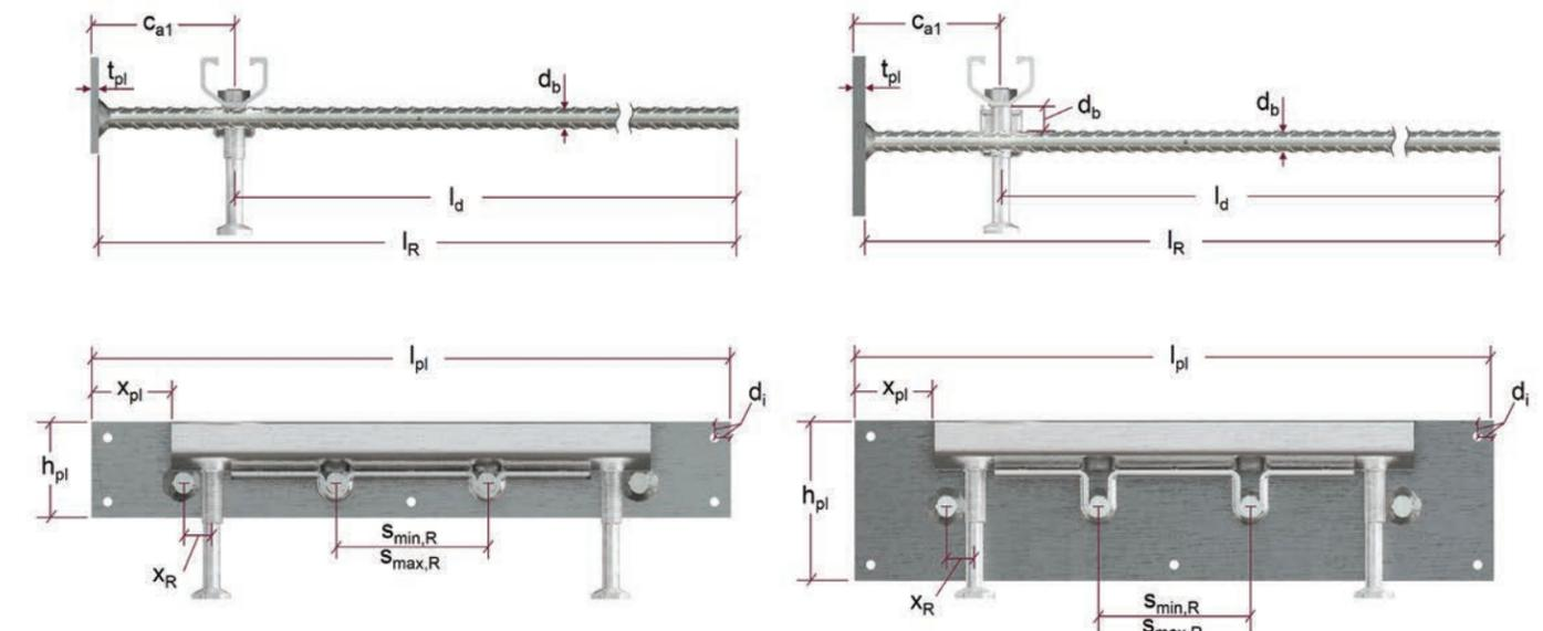
**Figure 2.2.7.8 – HAC EDGE Lite and HAC EDGE dimensions, section and elevation view.**
