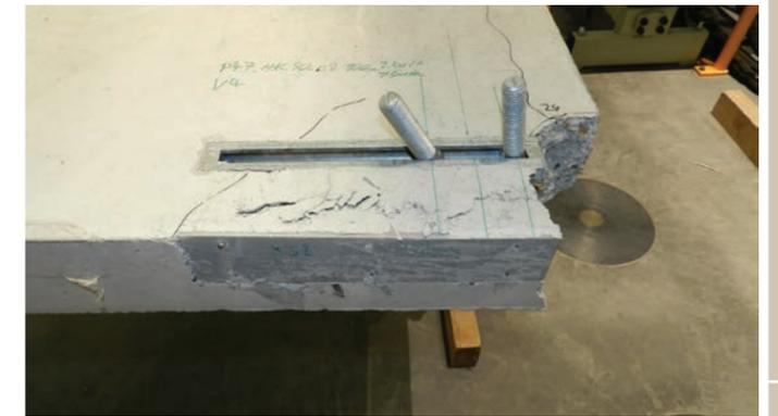
Figure 9.6.4.1 — HAC (T) EDGE, HAC (T) EDGE Lite or HAC S (T) EDGE — Side breakout in perpendicular shear when Anchor channel is installed at the corner.
