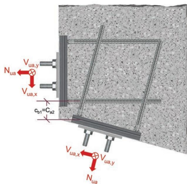
Figure 9.3.3.6 — HAC CRFOS U — Anchor channels on both sides - Obtuse angle Corner — Plan View.
