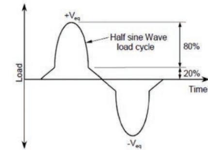
Figure 7.5.4.3 — Permitted approximation of seismic shear cycle (Figure taken from AC232, Figure 7.8).
