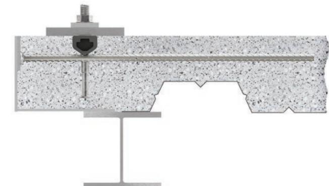
**Figure 2.2.16.17 — HAC-T EDGE in a composite slab, section view.**
