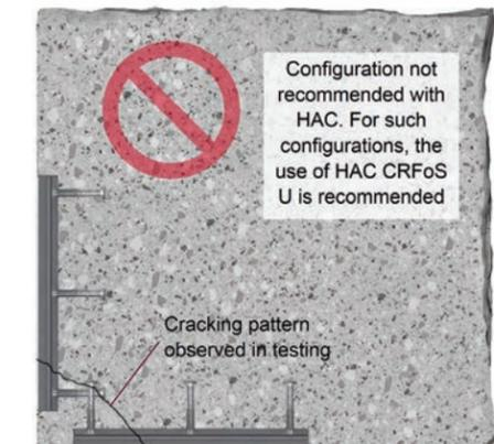
**Figure 2.2.14.3 — Premature concrete cracking due to simultaneous loading of pair HAC-T at corner with overlapped anchors, plan view.**
