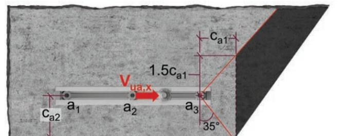
Figure 9.2.7.4 — Obtuse angle corner — TOS or BOS single channel at certain distance — Longitudinal Shear.
