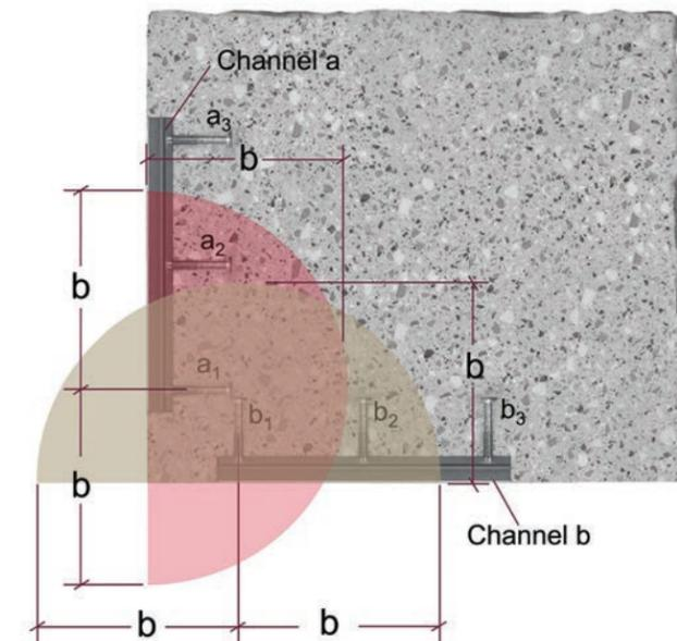
Figure 9.2.3.6 – 90° FoS corner with anchor channels on both sides –  $S_{cr,v}$ .
