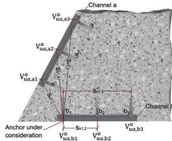
Figure 9.2.3.13 – Acute FoS corner with anchor channels on both sides – Example of determination of  $\psi_{s,v,a1}$ .
