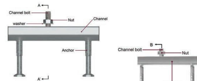
Elevation view of an anchor channel system.
