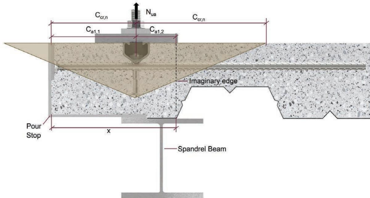
Figure 9.6.3.2 — HAC EDGE, HAC EDGE Lite and HAC S EDGE — Composite slab — Shear In.
