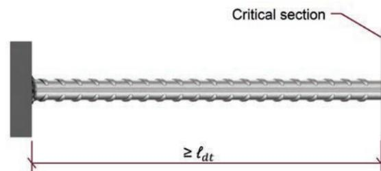
Figure 8.4.1.2 — Development length of headed anchored reinforcing bar.
