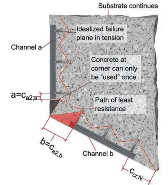
Figure 9.2.3.16 – Obtuse angle FoS corner with anchor channels on both sides – example of Tension analysis.
