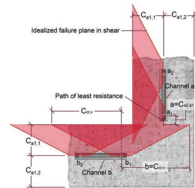
Figure 9.2.12.1-b — Inside Corner — Shear Perpendicular
