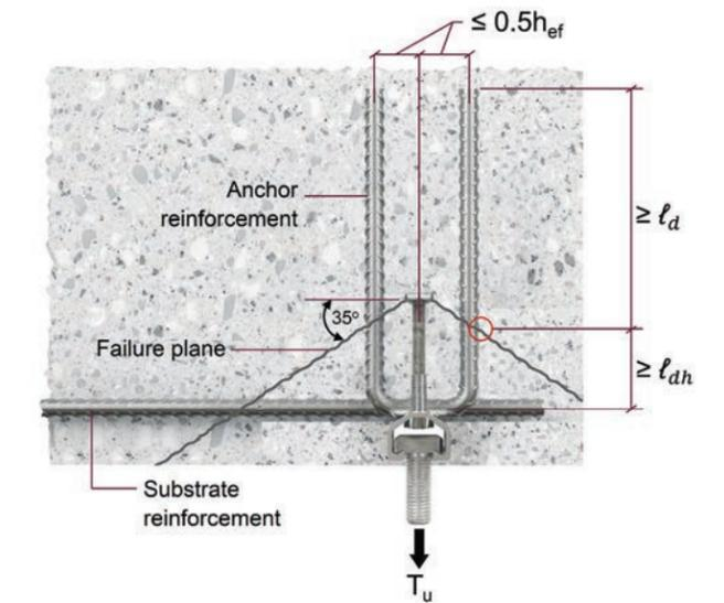
Figure 7.3.2.17 — Arrangement of anchor reinforcement for anchor channels loaded in tension, section view.
