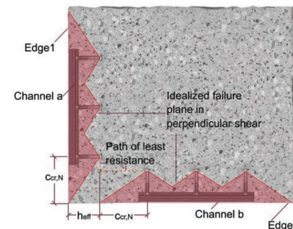
Figure 9.2.5.2— Minimum distance between anchor channels at the corner to assure the breakout cones do not intersect — Tension
