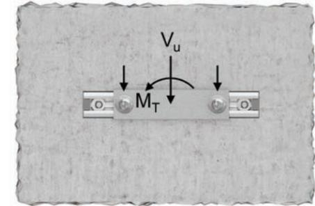
Figure 7.2.7.2 — Distribution of shear forces in an anchor group Example of connections in which all t-bolts participate in resisting the shear load.
