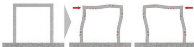
Seismic loading: cracks may occur almost everywhere in concrete members.
