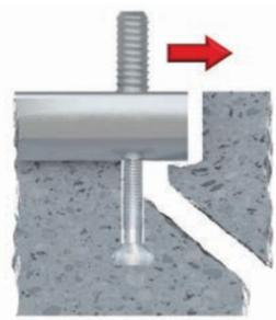
The nominal concrete breakout strength,  $V_{cb,x}$ , in shear acting in the longitudinal direction of an anchor channel in cracked concrete shall be computed as follows:
