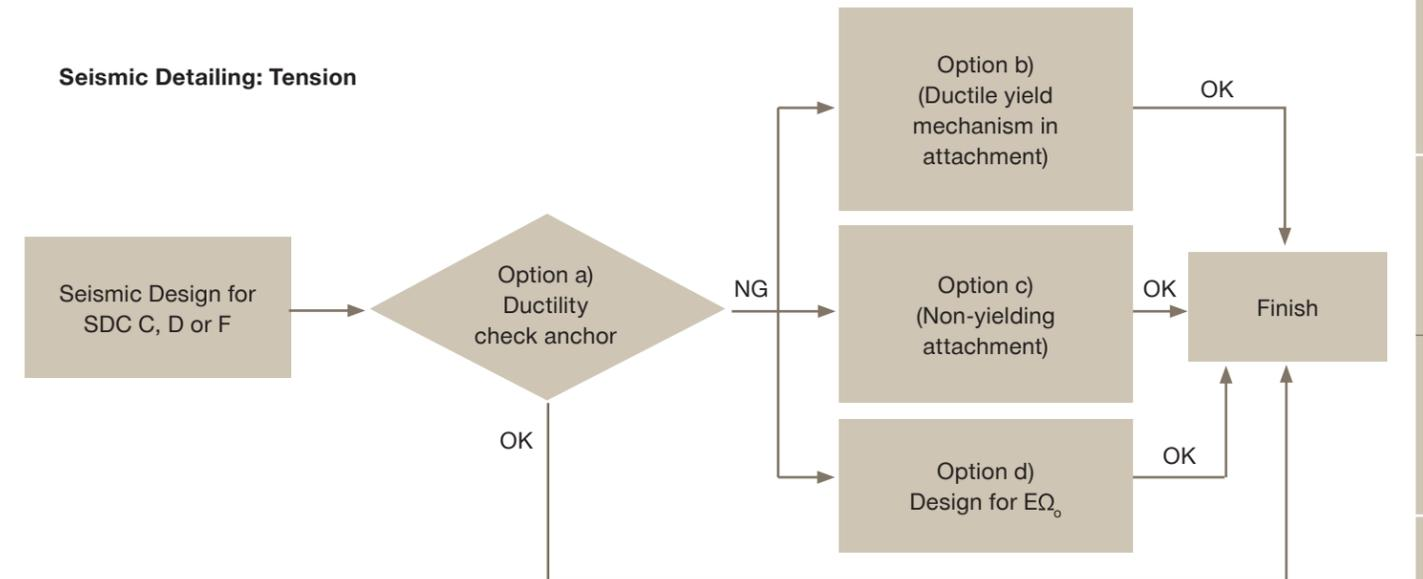
Figure 7.6.2.2 — Flow chart — Seismic provisions for tension; ACI 318-14 Section 17.2.3.4.3
