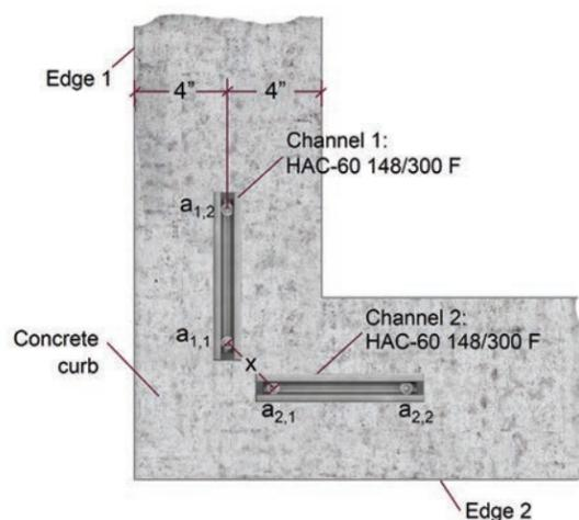
Figure 9.2.11.1 — Example of simplified method of HAC in a top of curb corner.
