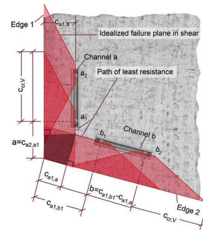
Figure 9.2.10.18-b — Simplified Method — Obtuse Corner — Perpendicular Shear
