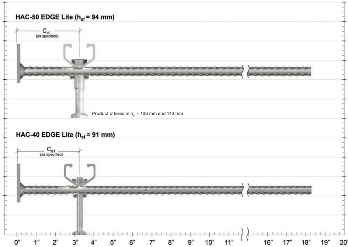
Figure 2.2.7.2 — Section view of HAC-40 EDGE Lite and HAC-50 EDGE Lite.
