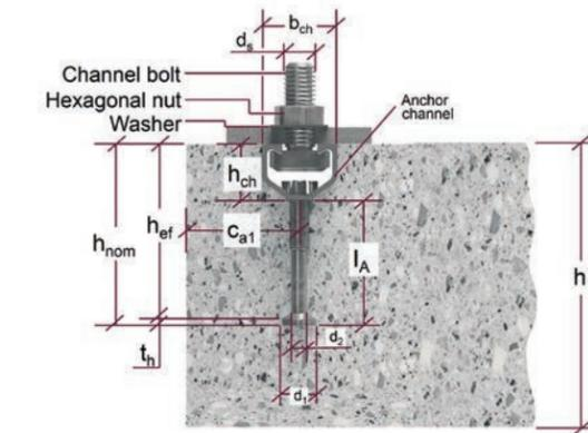
Cross-sectional view of an anchor channel system, A-A'.
