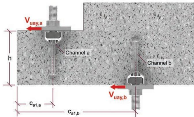
Figure 9.2.14.2 — Parallel Channels Top and Bottom: BOS away from TOS - Section View.
