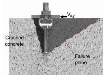
Figure 7.4.2.10 — Load-bearing mechanism of headed stud anchorage subjected to shear loading (schematic).
