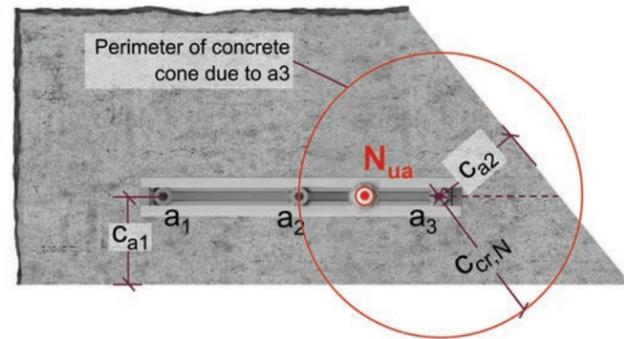
Figure 9.2.7.6 — Acute angle ToS corner with anchor channels on one sides — Tension.
