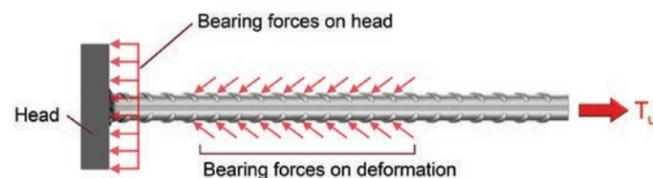
Figure 8.4.1.1 — Stresses on headed anchored reinforcing bars.
