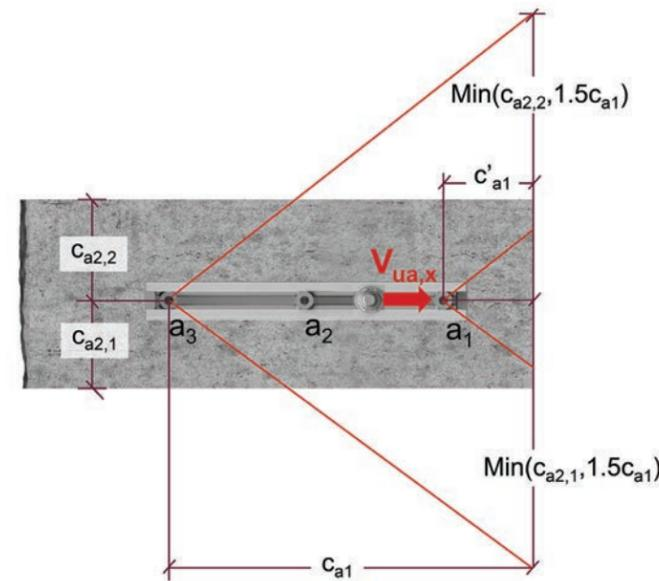
Figure 9.2.3.9 – 90° FoS corner with anchor channels on both sides – Effect of longitudinal, perpendicular shear and tension—section view
