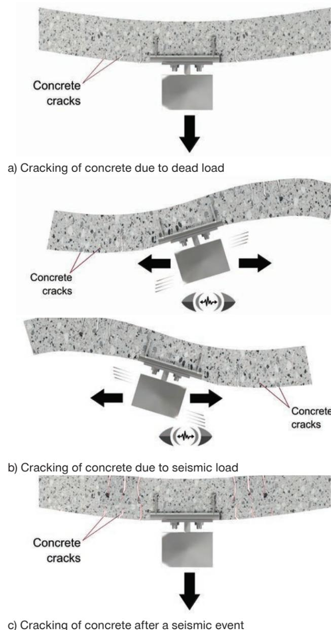
Figure 6.3.1 — Cracks in a reinforced concrete member subjected to cycling loads.
