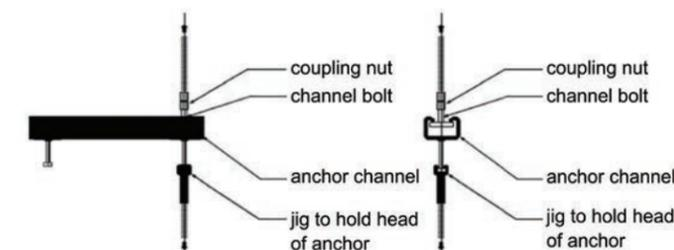
Figure 7.3.1.2 — Tension test setup for testing anchor channels in a universal testing machine. (Figure taken from AC232, Figure 5.5).
