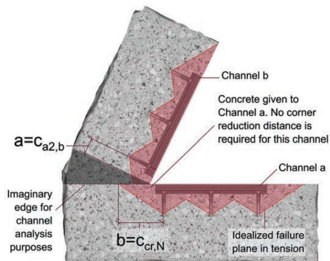
Figure 9.2.4.3— Acute angle interior FoS corner with anchor channels on both sides – Tension
