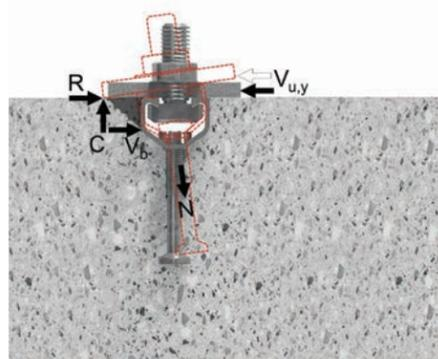
Figure 7.4.2.11 — Typical failure body of a stud anchorage far from an edge loaded in shear: Cross-section of failure body (schematic).
