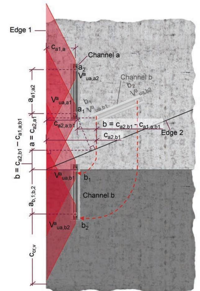
Figure 9.2.10.13b — Unfolding of Acute angle Corner.
