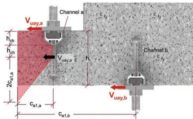
Figure 9.2.14.4— Parallel Channels Top and Bottom-BOS away from TOS: Perpendicular Shear TOS-Section View.
