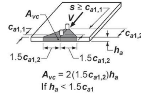
Figure 9.2.14.5—Calculation of  $A_{vc}$  for single anchors and groups of anchors per ACI 318-14.
