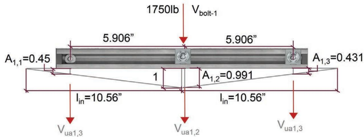
Figure 14.1.16 — Design example – effect of t-bolt 1 on anchors
