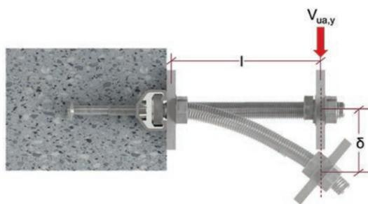
a)  $\alpha = 1$ ; fixture can rotate
