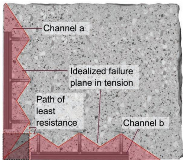
Figure 9.2.3.2 – 90° corner with anchor channels on both sides – overlapping of tension failure planes.
