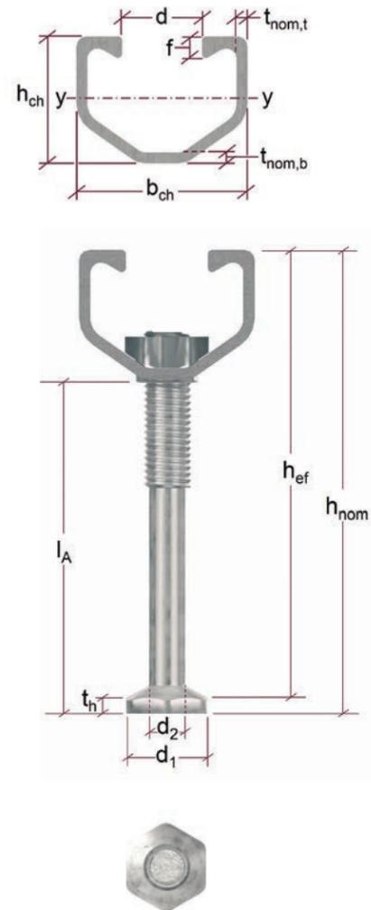
**Figure 2.2.7.5 a – Dimensions of the anchor channel of HAC EDGE Lite, HAC EDGE, and HAC S EDGE.**
