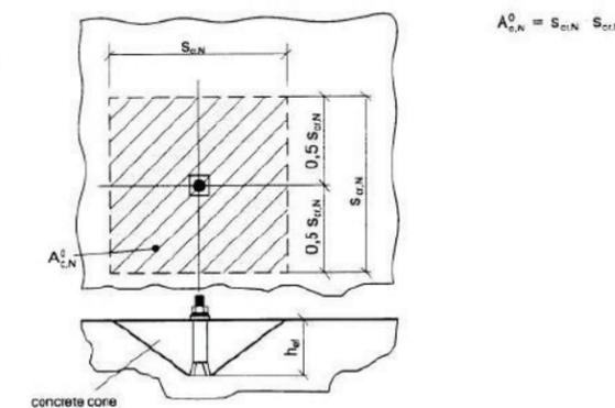
Figure 9.2.9.2 — ACI 318-14 - Fig. R17.4.2.1-(a) Calculation of  $A_{Ncc}$  per ACI318-14
