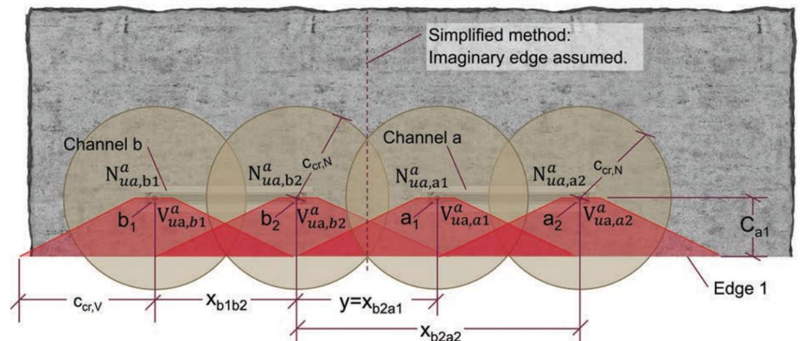
Figure 9.2.8.2 — TOS and BOS with pair of anchor channel adjacent to each other — Overlapping tension and perpendicular shear concrete cones.
