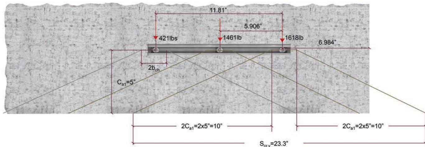
Figure 14.1.22 — Design example — spacing reduction factor of  $\psi_{s,v}$
