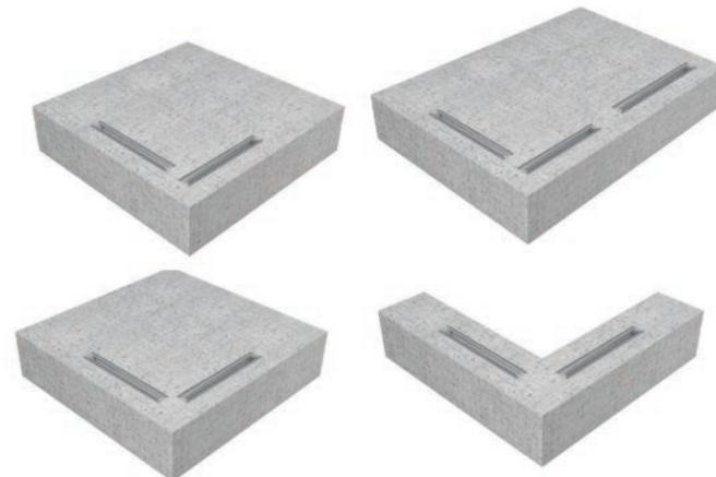
**Figure 2.2.15.3 — Corner configuration of pair of HAC-T or HAC-30 in top of slab.**
