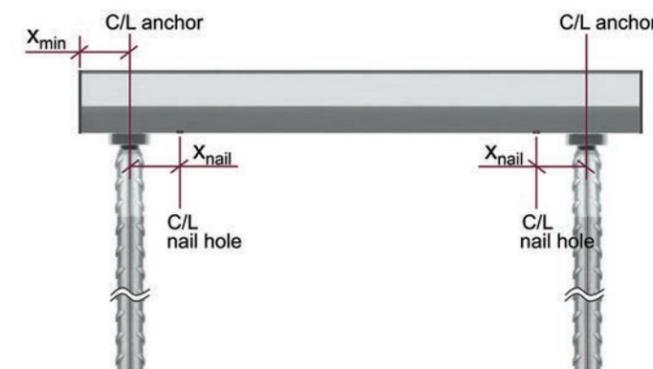
Figure 2.2.4.3 a — HAC CRFoS U end and nail hole distance.
