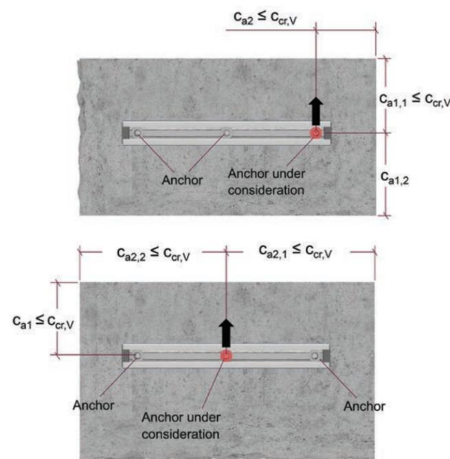
Figure 7.4.2.6 — Example of an anchor channel loaded in shear with anchors a) influenced by one corner and b) influenced by two corners.
