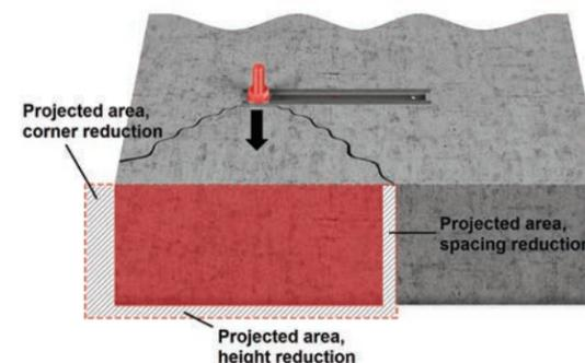
Figure 7.4.2.3 — Projected area of an anchor channel loaded in shear.
