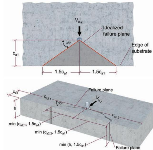
Figure 7.4.4.1 — Idealized failure planes and projected area of a cast-in anchor in accordance with ACI 318-14.
