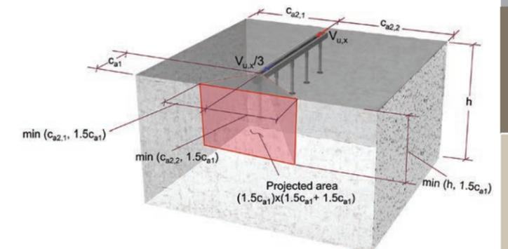
Figure 7.4.4.3 — Projected area due to an anchor channel loaded in shear acting parallel to the long channel axis. Shear forces acting on the leading anchor.
