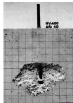
Figure 7.3.2.18 — Blowout failure of a deep anchor near an edge. (Picture from Anchorage in Concrete Construction, R. Elgehausen).
