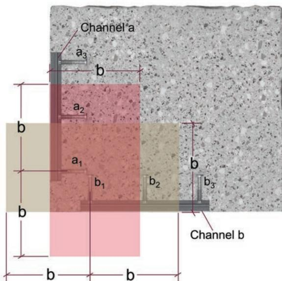
Figure 9.2.3.5 – 90° FoS corner with anchor channels on both sides – Effect of anchors closest to the edges.
