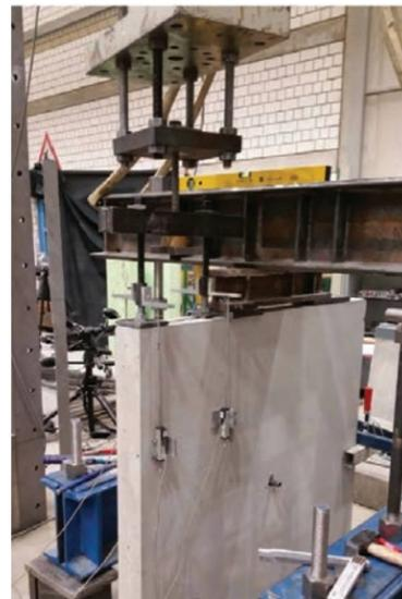
Figure 9.3.7 — Tension test setup for testing anchor channels under static and simulated seismic conditions.
