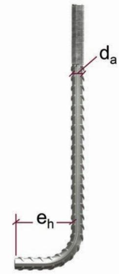
Figure 8.5.1.4 — L-reinforcing bar
