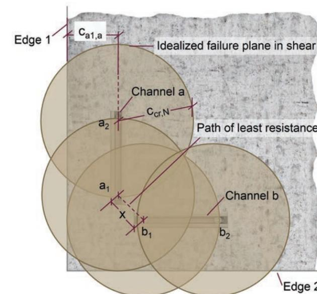
Figure 9.2.10.16-a— Simplified Method-90° Corner — Tension.
