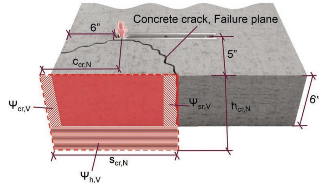
Figure 14.1.21 — Design example – reduction factors of  $V_{cb}$
