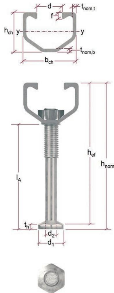
**Figure 2.2.16.5 a — Dimensions of the anchor channel of HAC-T EDGE Lite, HAC-T EDGE, and HAC-T S EDGE.**
