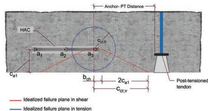
Figure 11.5.3.2 — Top of slab configuration with live end of post-tensioned slab outside the anchorage zone.
