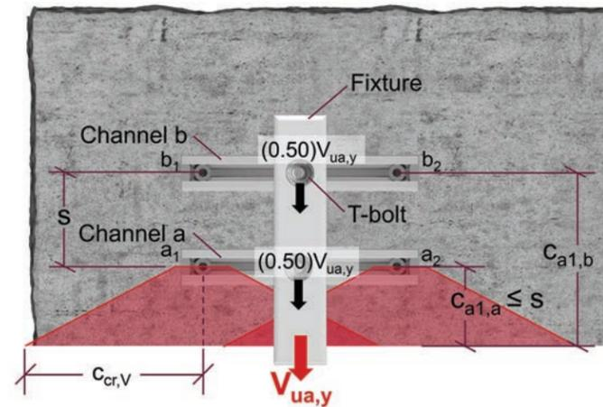
Figure 9.2.13.2 — Parallel Channels-Perpendicular Shear Casel-Plan.
