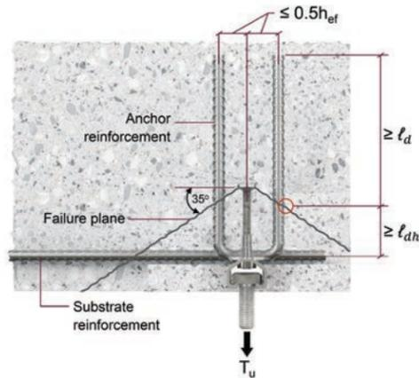
Figure 7.3.2.3 — Arrangement of anchor reinforcement for anchor channels loaded by tension load at an edge.
