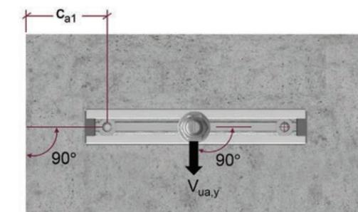
Figure 7.4.2.4 — Anchor channel arranged perpendicular to the edge and loaded parallel to the edge.
