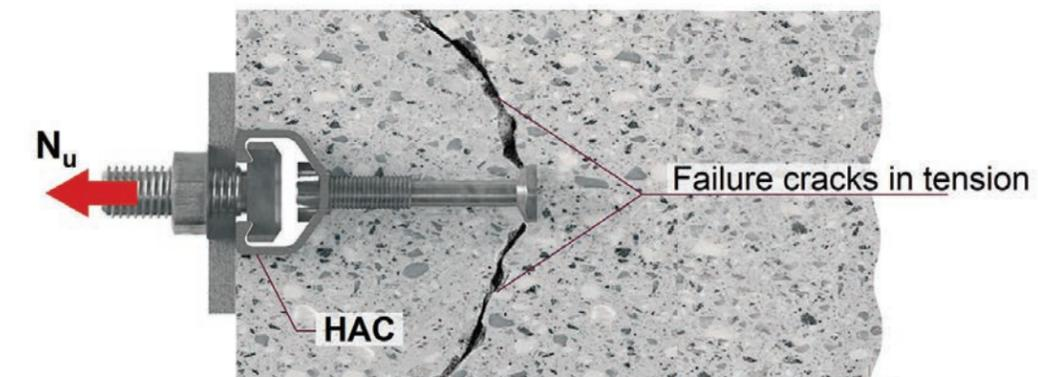
Figure 9.3.1 — Concrete breakout in tension of a cast-in anchor channel with rounded stud head anchors (HAC) — Section View.
