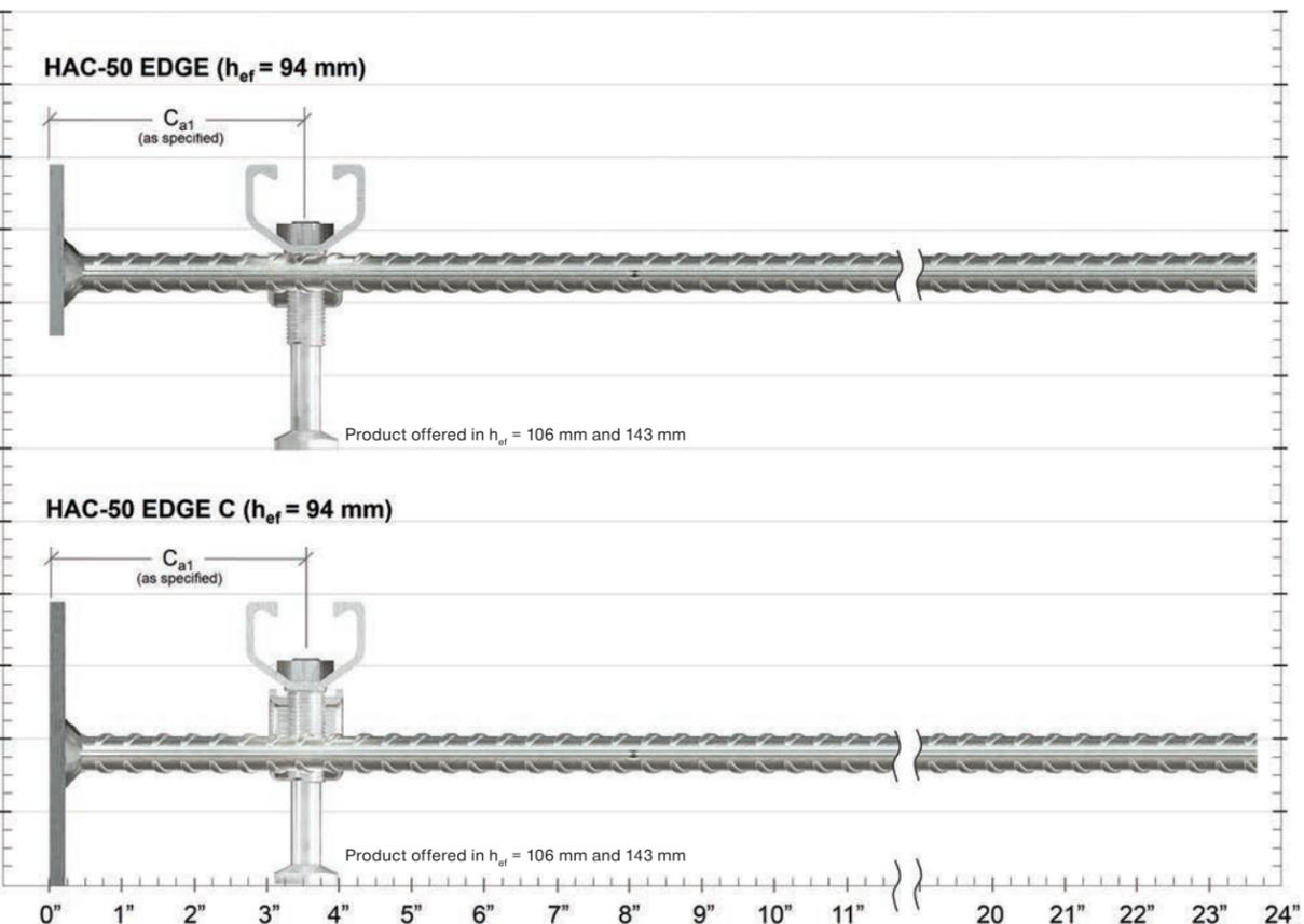
Figure 2.2.7.3 — Section view of HAC-50 EDGE and HAC-50 EDGE C.
