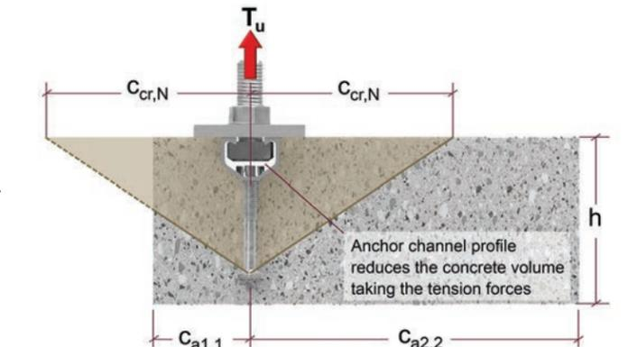
Figure 7.3.2.7 — Concrete Breakout cone in tension
