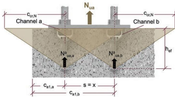
Figure 9.2.13.7 – Tension - Equal tension force-Section view.
