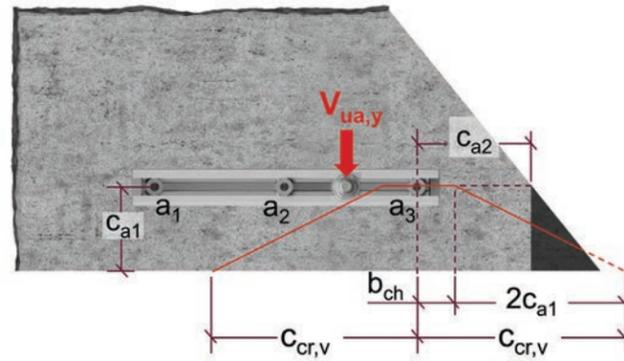
Figure 9.2.7.5 — Acute angle ToS corner with anchor channels on one sides — Perpendicular shear.
