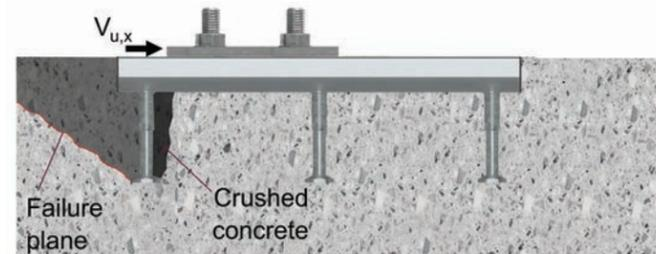
Figure 7.4.4.7 — Load-bearing mechanism of headed stud anchorage subjected to shear loading (schematic).
