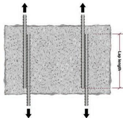
Figure 8.6.1.4 — Contact lap splice.
