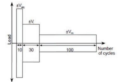
Figure 7.5.4.2 — Required load history for simulated seismic shear test (Figure taken from AC232, Figure 7.7).
