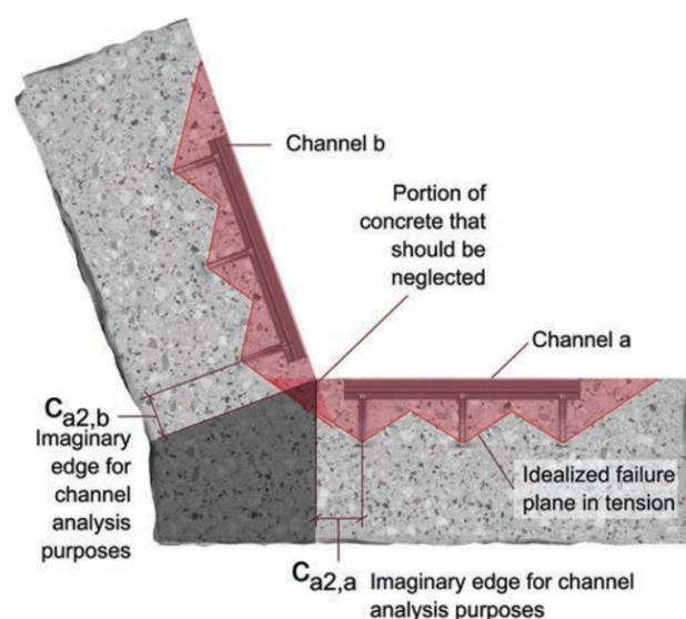
Figure 9.2.4.5 — Obtuse angle interior FoS corner with anchor channels on both sides.
