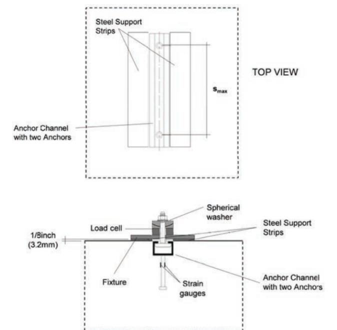
Figure 7.3.1.3 — Test setup for tests in accordance with table 4.1 of AC232, test No. 5. (Figure taken from AC232, Figure 7.1)
