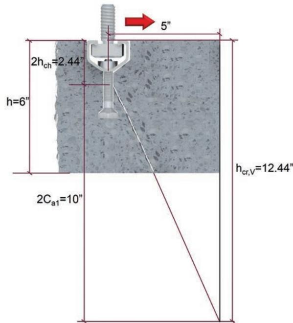
Figure 14.1.24 — Design example – height reduction factor  $h_{cr,w}$
