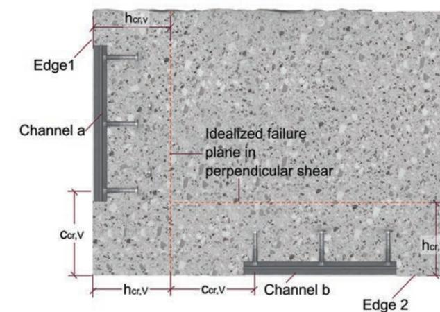
Figure 9.2.5.1— Minimum distance between anchor channels at the corner to assure the breakout cones do not intersect — Tension
