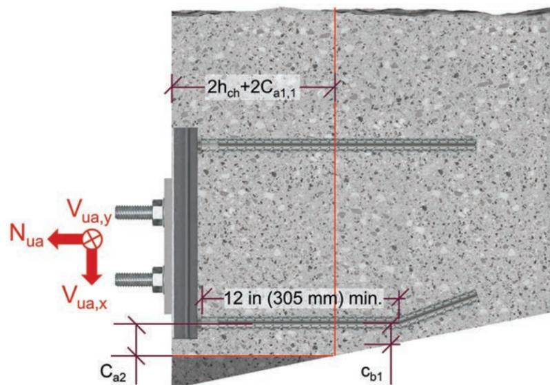
Figure 9.3.2.2 — HAC CRFOS U — Single anchor channel — Acute angle Corner — Plan View.
