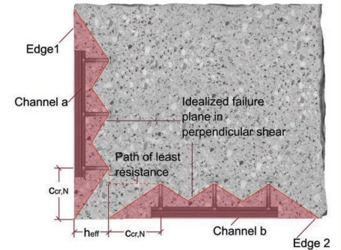
Figure 9.2.3.1 — 90° corner with anchor channels on both sides — Failure planes does not intersect.
