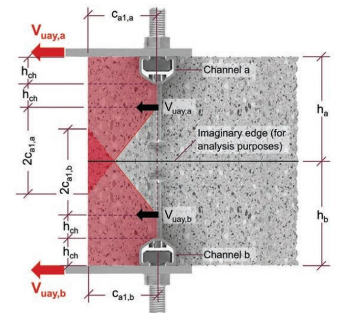
Figure 9.2.14.12 — Top and Bottom Channel: TOS under BOS -Perpendicular Shear — Section View.
