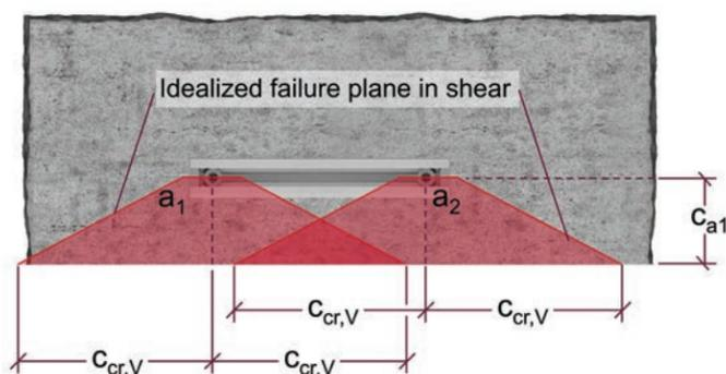
Figure 9.2.10.11a — Single anchor channel in shear.
