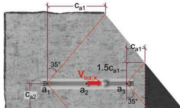
Figure 9.2.7.7 — Acute angle ToS corner with anchor channels on one sides — Longitudinal shear.
