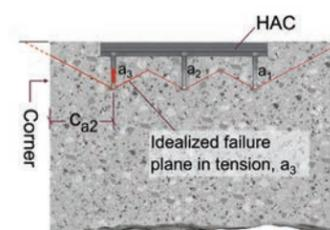
Figure 9.2.2.1: 90° Corner with single channel.
