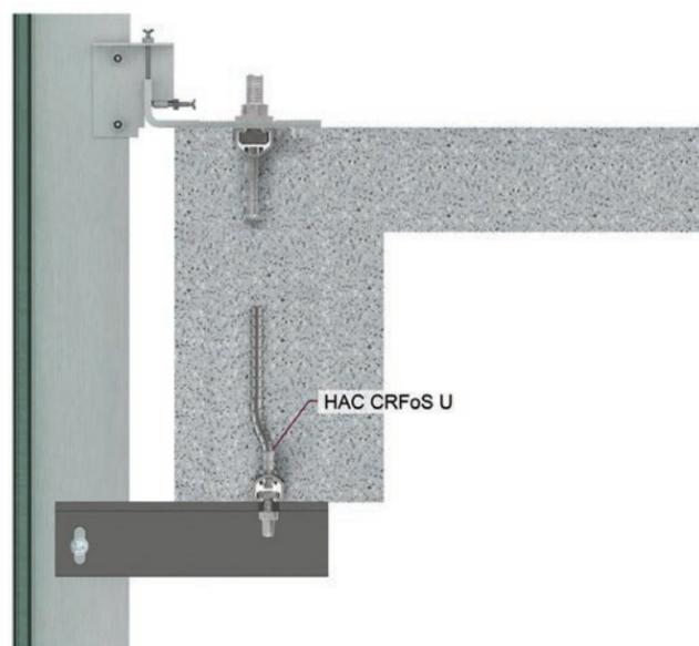
Figure 2.2.6.2 — HAC CRFoS U in bottom of slab application, section view.
