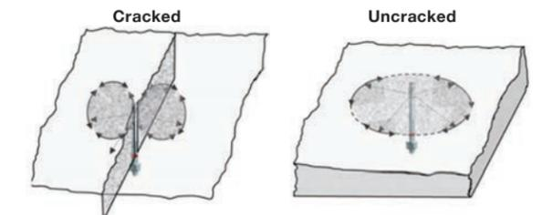
Figure 7.3.2.2 — Concrete cone in cracked (left) and uncracked (right) concrete.
