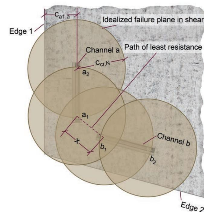
Figure 9.2.10.18-a — Simplified Method — Obtuse Corner — Tension .
