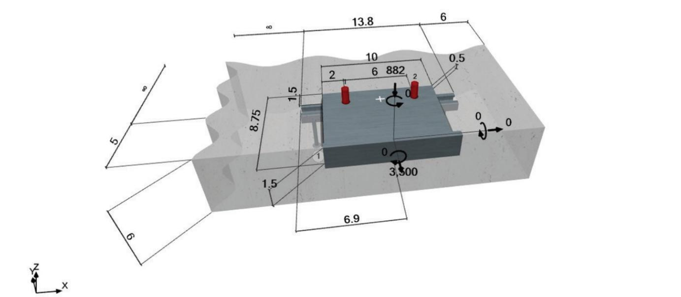
Figure 14.1.10 — Design example – Profis anchor channel - 3D Front View
