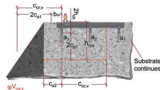
Figure 9.2.2.4 — Obtuse corner — perpendicular shear — Section view.
