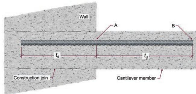
Figure 8.2.1.2 — Development length of a reinforcing bar in a cantilever member. Source: Wight, James & MacGregor, James. Reinforced Concrete Mechanics & Design, 2012.
