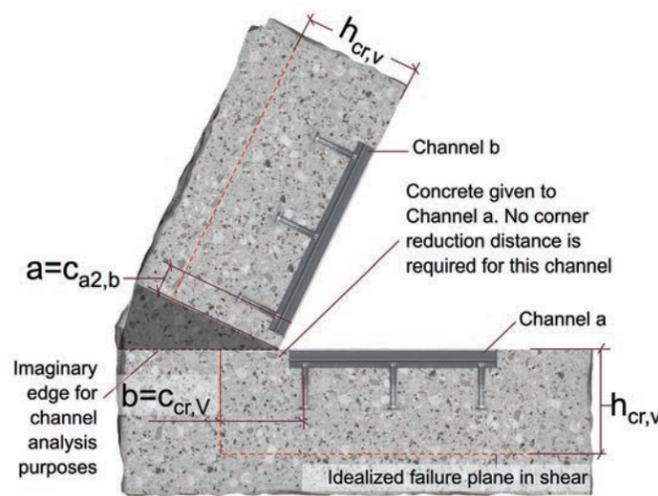
Figure 9.2.4.4 — Acute interior FoS corner with anchor channels on both sides — Perpendicular shear
