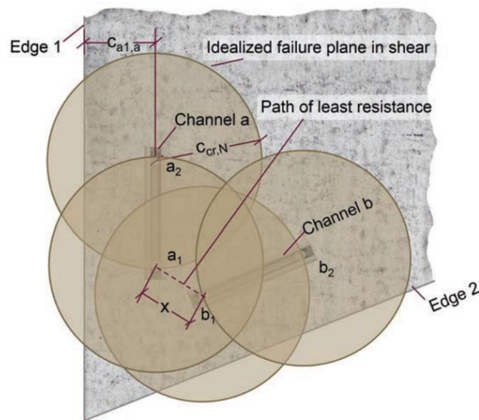
Figure 9.2.10.17-a — Simplified Method — Acute Corner — Tension.
