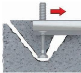
Failure load associated with pry-out; The load-bearing mechanism of a single headed stud anchorage subjected to a shear load is illustrated schematically in Figure 7.4.47. The applied shear load gives rise to bearing stresses in the concrete. With increasing load, the surface concrete is crushed or spalled, shifting the centroid of resistance  $V_b$  to a location deeper in the concrete.
