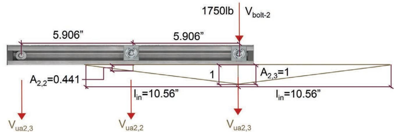
Figure 14.1.17 — Design example – effect of t-bolt 2 on anchors
