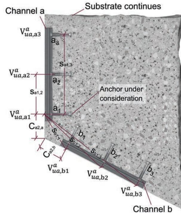
Figure 9.2.3.16.17— Obtuse FoS corner with anchor channels on both sides —Example of determination of  $\psi_{s,v,a1}$ .
