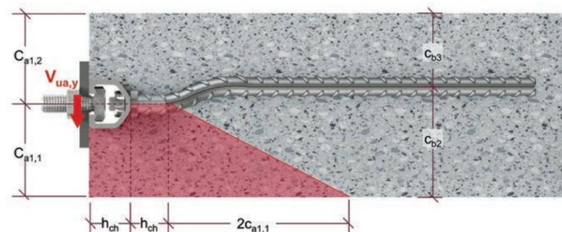
Figure 9.3.2.3 — HAC CRFOS U — Single anchor channel — Acute angle Corner — Section View.
