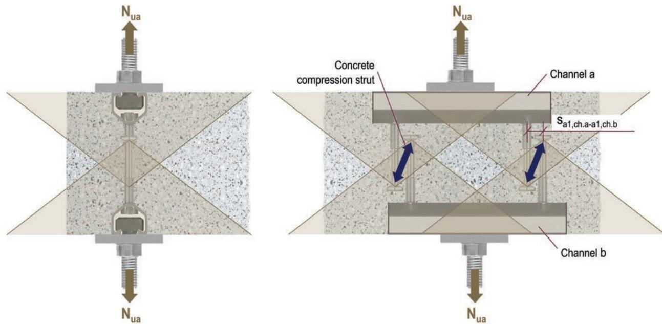
Figure 9.2.14.13 — Intersecting Top and Bottom Channel; tension loading
