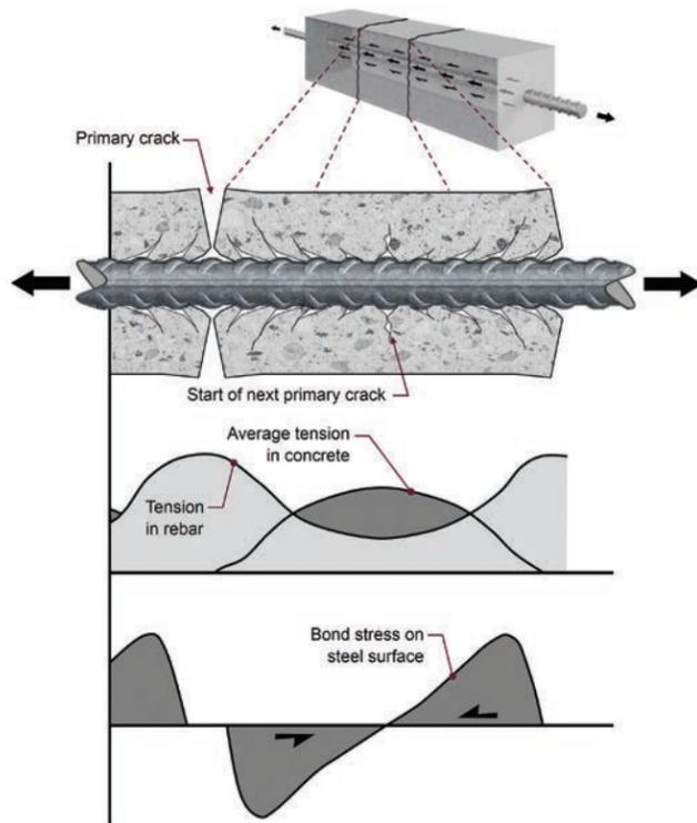
Figure 8.2.1.1 — Stresses in concrete and rebar.
