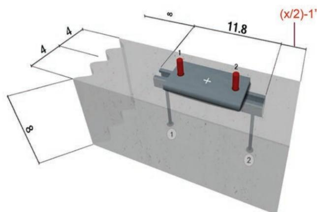
Figure 9.2.11.2 — Analysis of channel 1 using the simplified method in PROFIS Anchor Channel.
