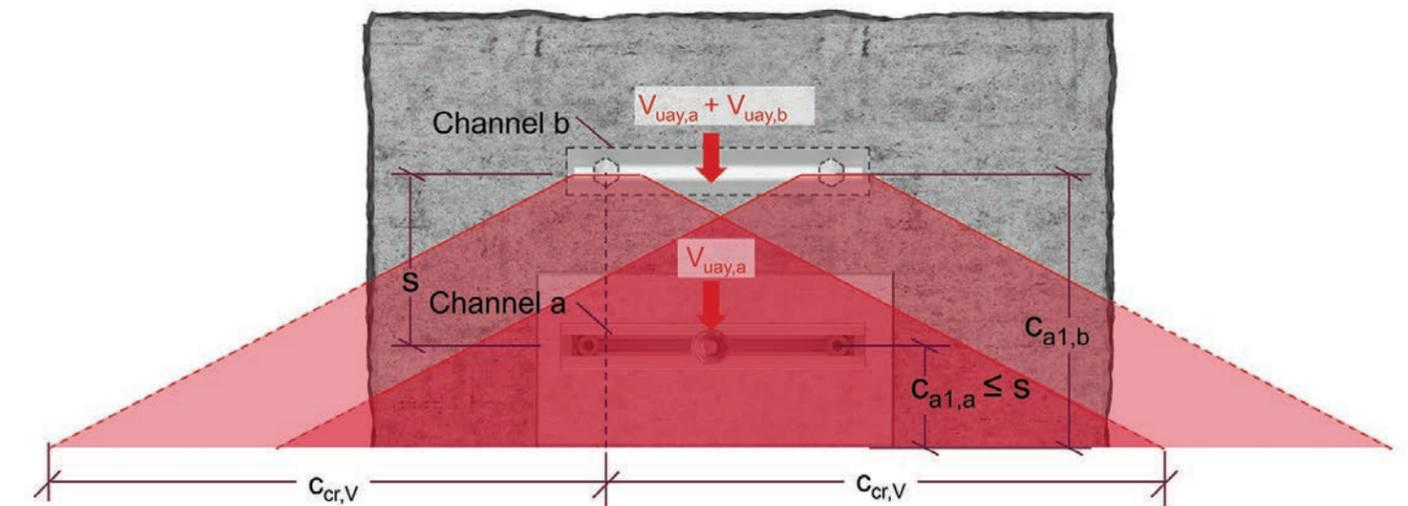
Figure 9.2.14.7 — Parallel Channels Top and Bottom: BOS away from TOS-Perpendicular Shear BOS-Plan View.
