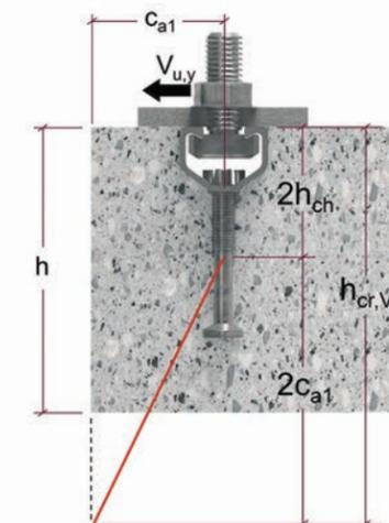
Figure 7.4.2.7 — Example of an anchor channel in a member with a thickness  $h < h_{cr,V}$
