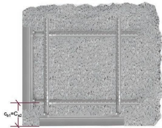
Figure 9.3.3.1 — HAC CRFOS U — Anchor channels on both sides — 90 degree angle Corner — Plan View.
