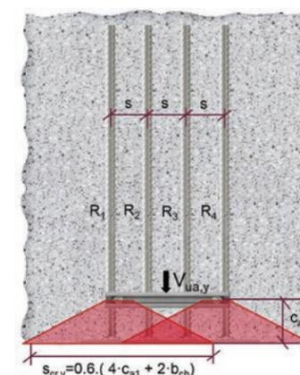
Figure 9.6.2.5 – Modification of anchor spacing:  $\Psi_{s,v}$
