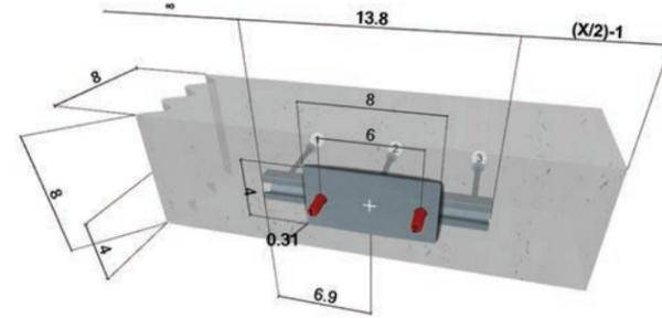
Figure 9.2.6.2 — Example of use of HAC-40 91/300 F on a curb installing the anchor channel Face of curb.
