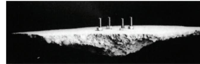
Figure 7.3.2.6 — Concrete cone breakout of a group of anchors. (Picture from Anchorage in Concrete Construction, R. Eligehausen).
