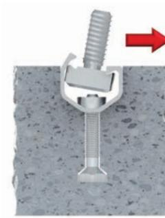
The nominal strength of the channel lips to take up shear loads perpendicular to the channel transmitted by a channel bolt, V<sub>sl,y</sub>, must be taken from Table 8-5 for HAC and HAC-T with Hilti channel bolts (HBC-B, HBC-C, HBC-T and HBC-C-N).
