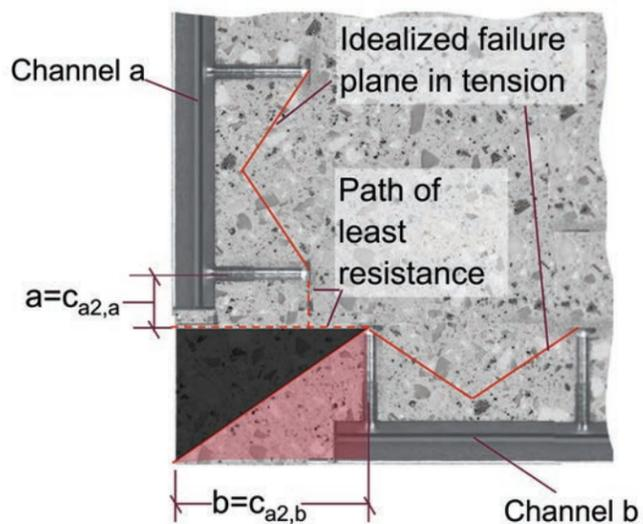
Figure 9.2.3.3 – 90° corner with anchor channels on both sides – Detail showing the edge distance that needed be used in analysis.
