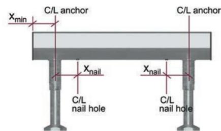
**Figure 2.2.7.5 b – HAC end and nail hole distance.**
