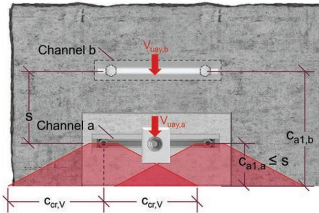
Figure 9.2.14.3 — Parallel Channels Top and Bottom: BOS away from TOS-Perpendicular Shear TOS-Plan View.
