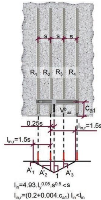
Figure 9.6.2.9 — Example for the calculation of rebar forces in accordance with the triangular load distribution method for an anchor channel with four rebars. The influence length is assumed as  $\ell_{in} = 1.5s$
