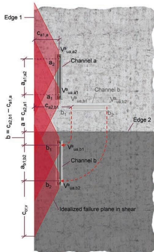
Figure 9.2.10.12b — Unfolding of 90° Corner.
