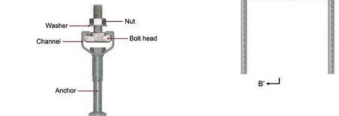
Cross-sectional view of an anchor channel system, A-A'.
