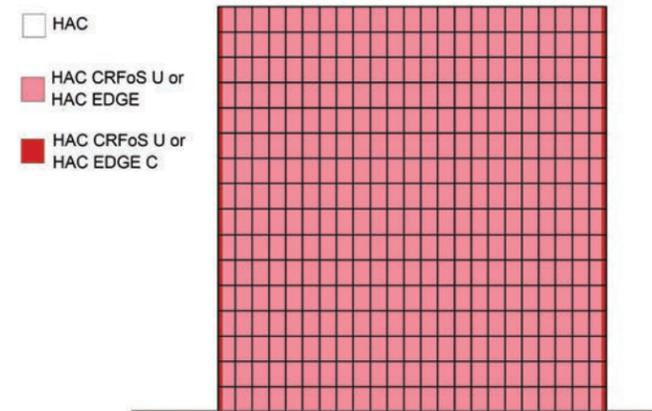
Figure 11.4.1.3 Typical anchor channel layout for composite slabs
