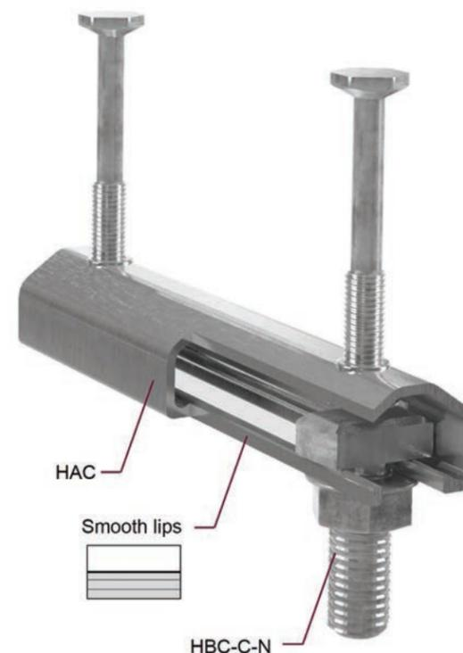
Figure 7.6.4.1: Standard HAC channel with locking t-bolt HBC-C-N.
