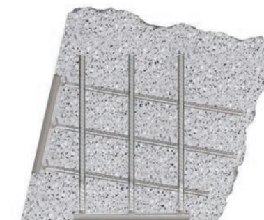
Figure 2.2.5.4 — Pair of HAC CRFoS U in an acute corner, plan view.
