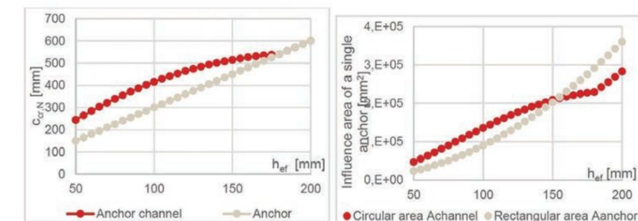
Figure 9.2.9.3 — Comparison of  $C_{cr,N}$  for anchors and for an anchor channels (left), Comparison of the idealized breakout area for anchors and for an anchor channel (right)
