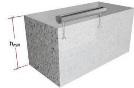
Figure 2.2.1.5 – Minimum HAC member thickness, isometric view.
