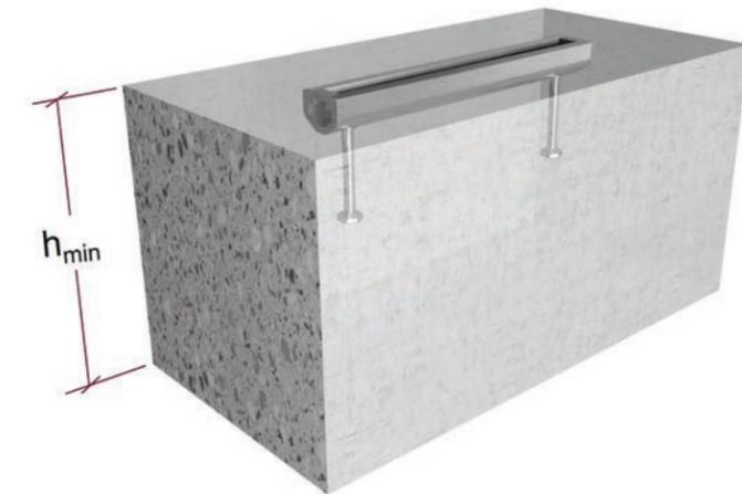
**Figure 2.2.13.7 — Minimum HAC-T and HAC-30 member thickness, isometric view.**
