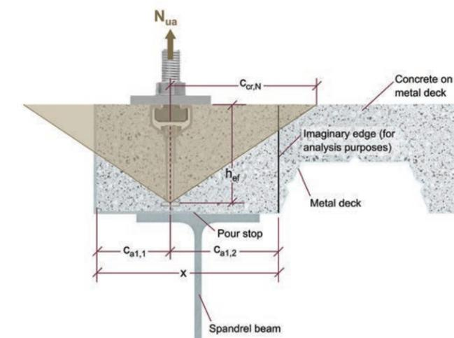
Figure 9.2.15.2 — TOS: Composite Slab — Tension — Section View.
