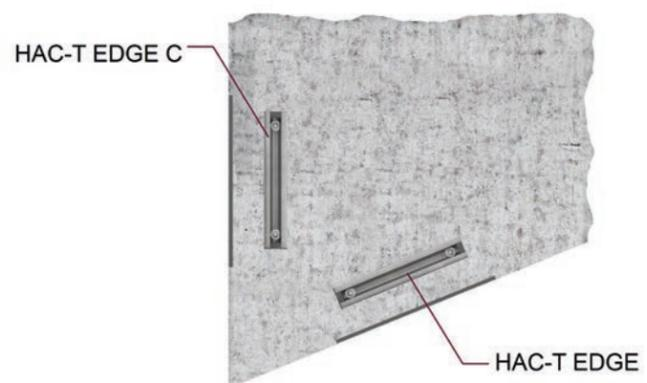
Figure 2.2.17.3 — HAC-T EDGE and HAC-T EDGE C in an acute corner, plan view.
