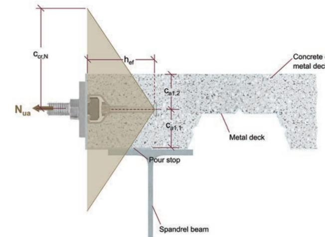
Figure 9.2.15.1 — FOS: Composite Slab — Tension — Section View.
