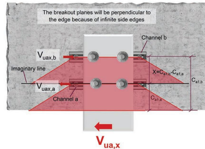
Figure 9.2.13.10 – Longitudinal Shear – Plan view.
