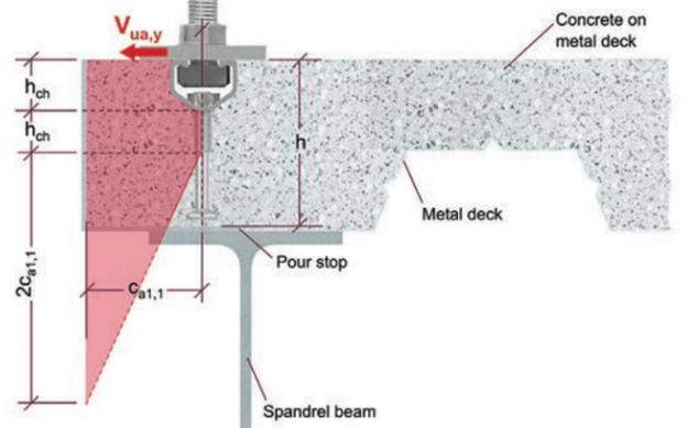
Figure 9.2.15.2-b — TOS: Composite Slab — Perpendicular Shear — Section View.
