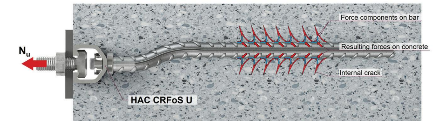
Figure 9.3.2 — Concrete failure mode of Cast-in anchor channel with rebar anchors (HAC CRFoS U) — Section View.
