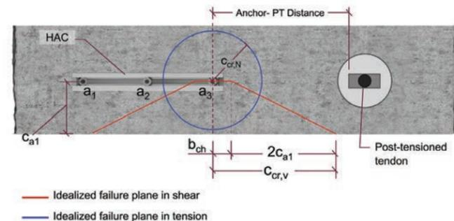
Figure 11.5.3.1 — Face of slab configuration with live end of post-tensioned slab outside the anchorage zone.
