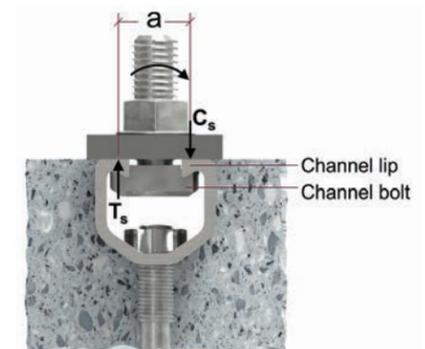
Figure 7.4.1.2 - Definition of internal lever arm.
