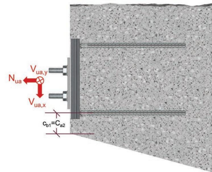
Figure 9.3.2.4 — HAC CRFOS U — Single anchor channel — Obtuse angle Corner — Plan View.
