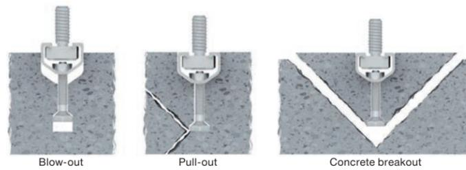
Figure 7.6.2.3 — Tensile anchor channel failure modes with an additional 0.75 reduction strength when resisting earthquake forces
