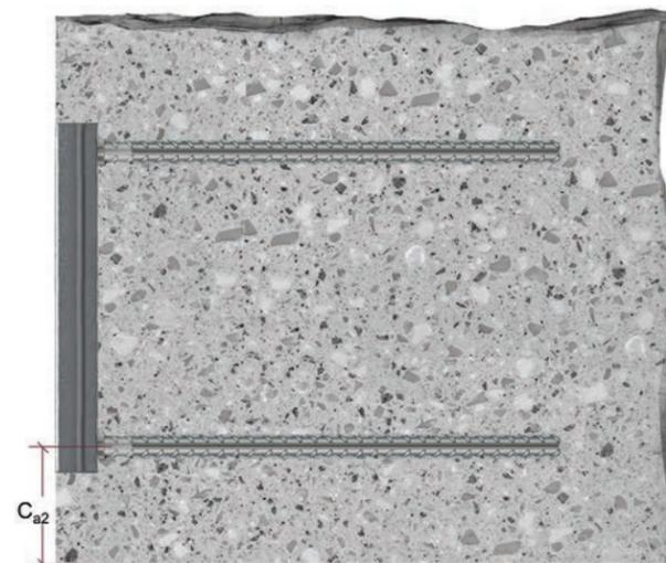
Figure 9.3.2.1 — HAC CRFOS U — Single anchor channel — 90 degree Corner.
