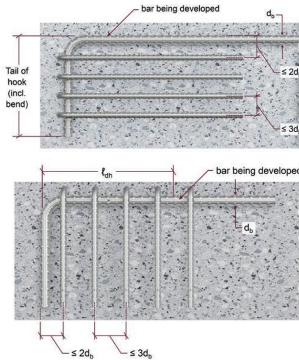
Figure 8.5.1.3 — Confinement of hooks by stirrups and ties. Source: Wight, James & MacGregor, James. Reinforced Concrete Mechanics & Design, 2012.
