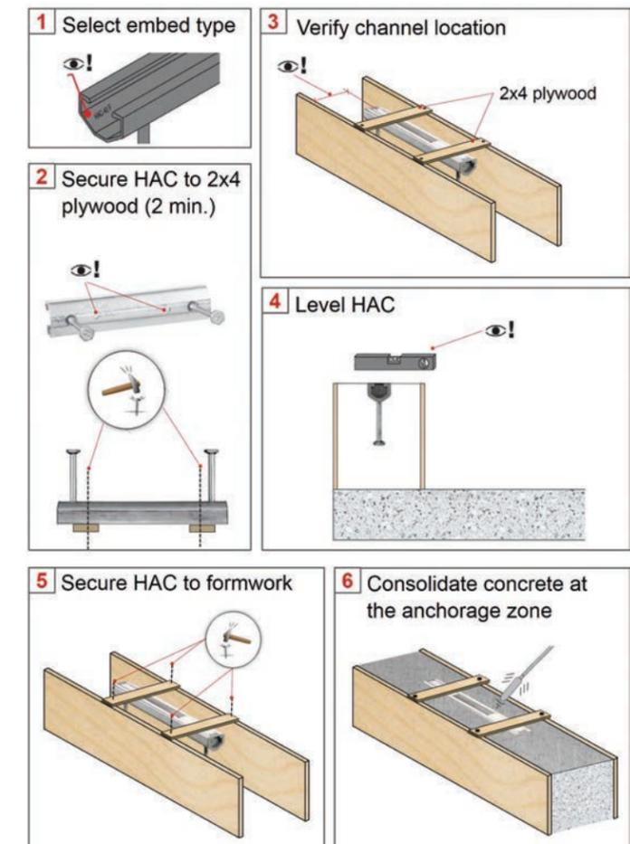
Figure 11.5.5.1 — Installation of HAC in top of slab curbs.
