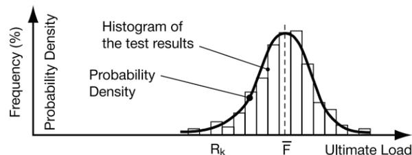
Fig. 5.2.1 Frequency distribution of anchor ultimate loads, demonstrating the significance of the 5% fractile
