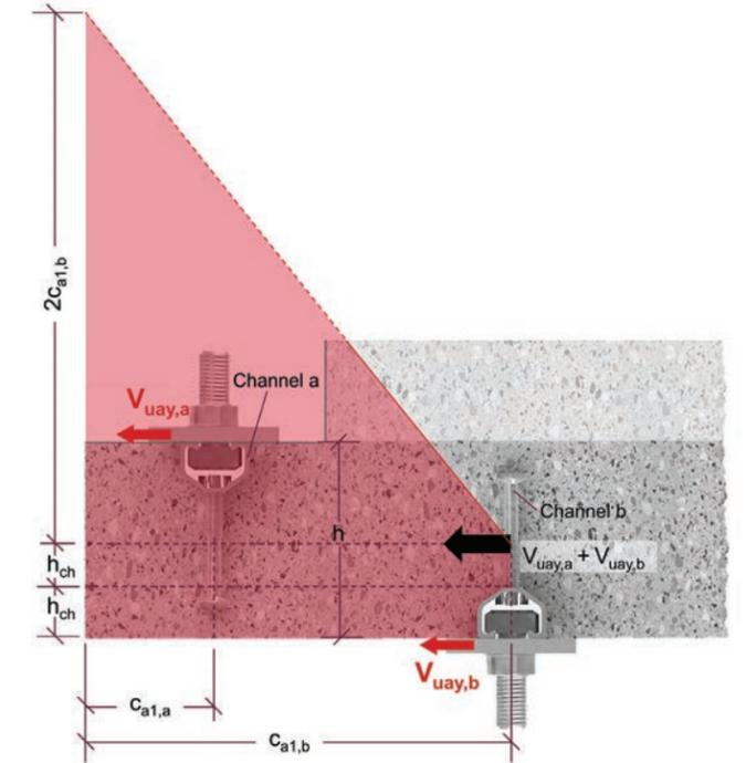
Figure 9.2.14.6 — Parallel Channels Top and Bottom: BOS away from TOS-Perpendicular Shear BOS Section View.
