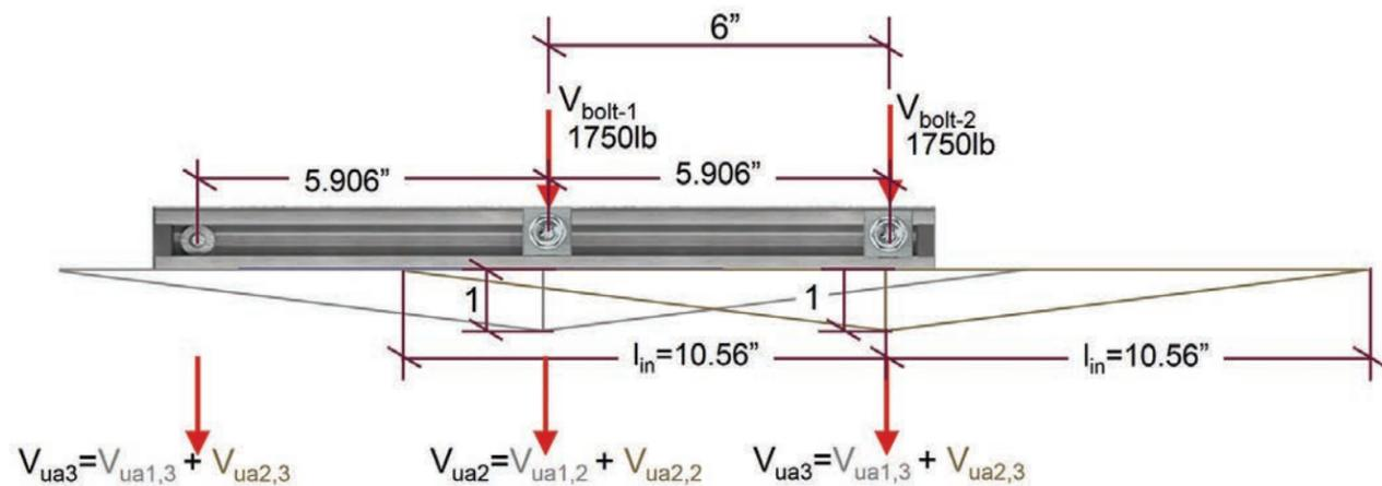
Figure 14.1.18 — Design example – Anchor Shear forces
