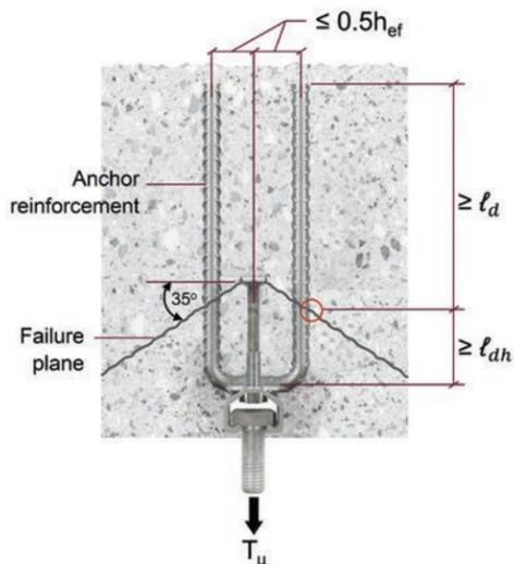
Figure 7.3.2.4 Arrangement of anchor reinforcement for anchor channels loaded by tension load in a narrow member.
