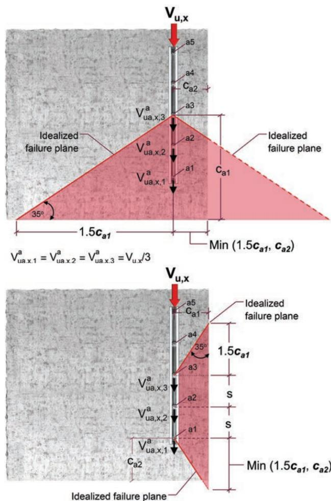
Figure 7.2.8.5 — Example for the calculation of anchor channels with 6 anchors loaded in shear longitudinal to the channel axis for concrete edge failure.
