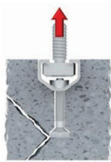
Tension-loaded headed studs provided with small edge distances can generate local blowout failures in the vicinity of the head. Side blow-out failure will govern the concrete capacity of studs having small edge distance (concrete cover) in combination with large embedment depth. Local concrete side blow-out failure is caused by the quasi-hydrostatic pressure in the region of the head of the stud which gives rise to a lateral bursting force. The failure
