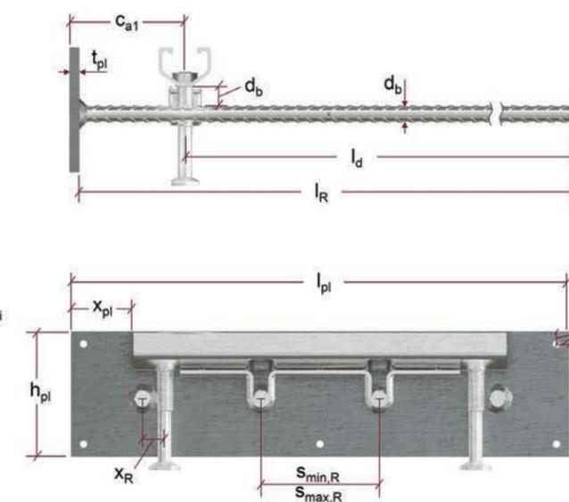
**Figure 2.2.16.9 — HAC-T EDGE C dimensions, section and elevation view.**
