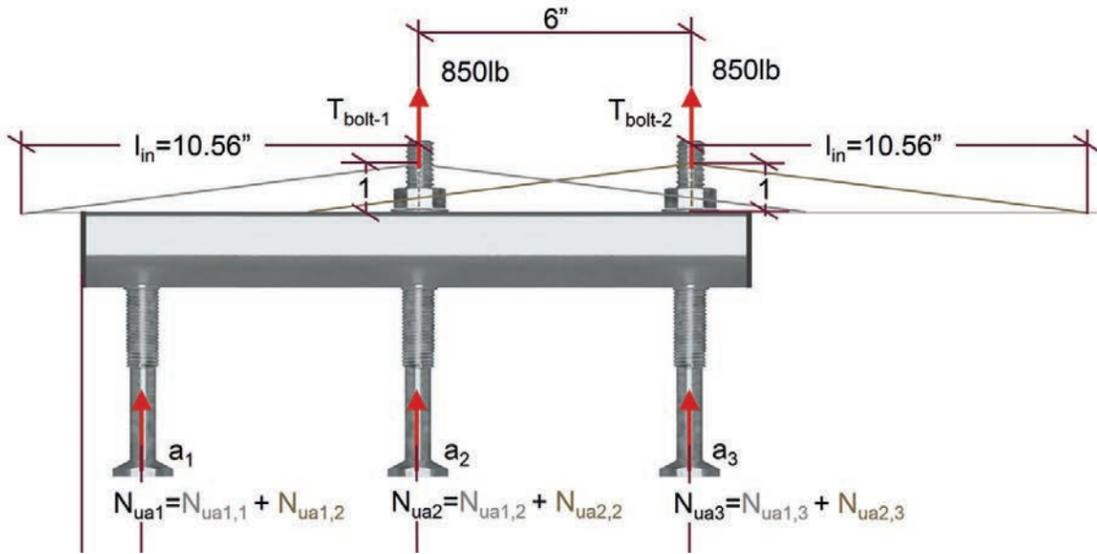
Figure 14.1.14 – Design example – Anchor Tension forces
