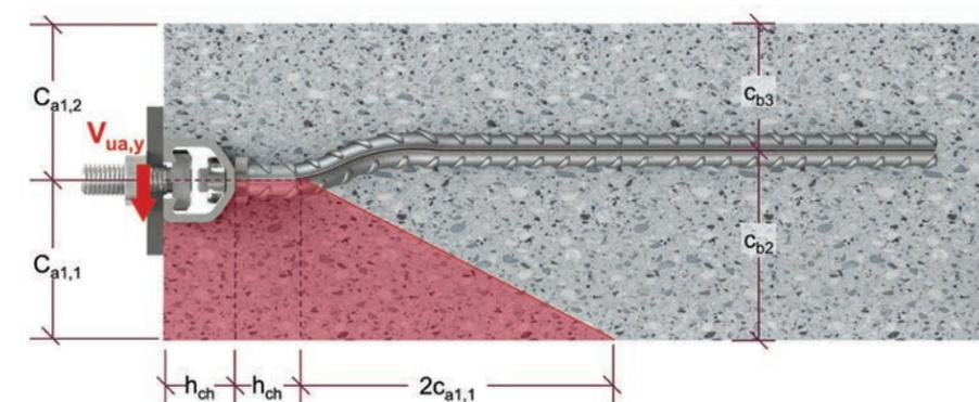
Figure 9.3.2.5 — HAC CRFOS U — Single anchor channel — Obtuse angle Corner — Section View.
