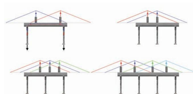
Figure 7.2.8.2 — Triangular load distribution for different anchor channel system configurations.
