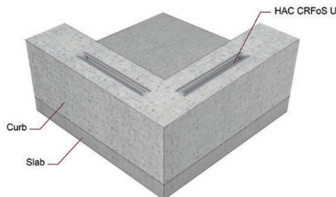
Figure 2.2.6.1 — Pair of HAC CRFoS U in a top of curb corner, isometric view.
