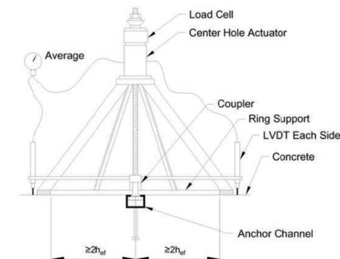
Figure 7.3.1.4 — Example of an unconfined tension test setup for testing anchor channels (Figure taken from AC232, Figure 5.4).
