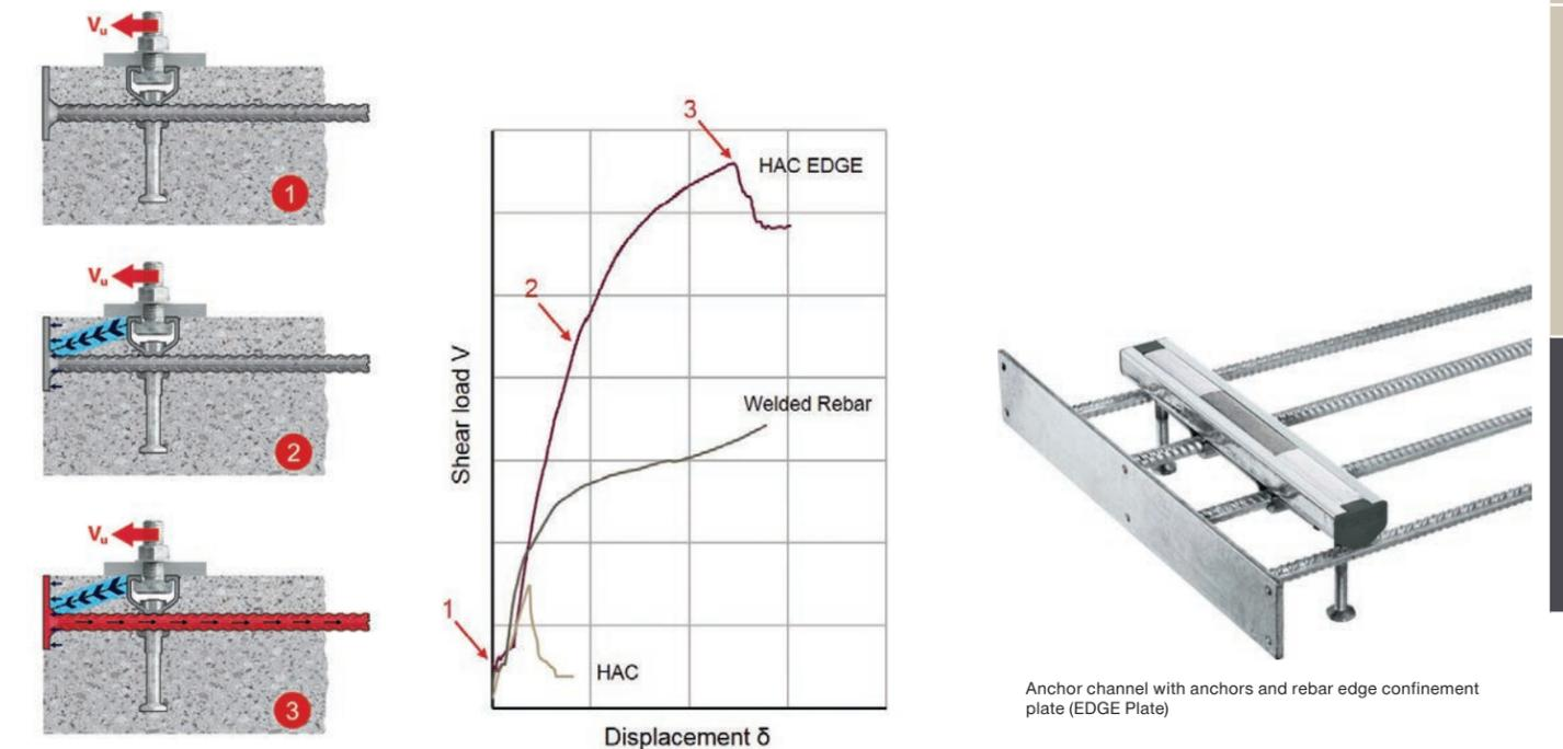
Figure 9.6.1.5 — HAC EDGE Behavior of HAC EDGE loaded in shear (left). Shear load vs displacement curve (right).
