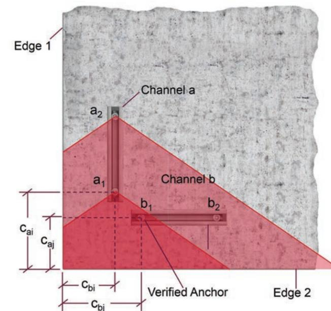
Figure 9.2.10.15 — Interacting tension with perpendicular shear and longitudinal shear.
