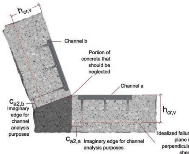
Figure 9.2.4.6 — Obtuse angle interior FoS corner with anchor channels on both sides —perpendicular shear
