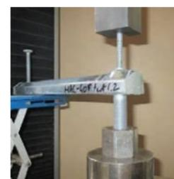
Figure 9.3.6-b — Tension test setup universal testing machine.
