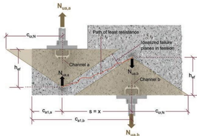
Figure 9.2.14.8 — Parallel Channels Top and Bottom-BOS away from TOS: Tension- TOS and BOS Section View.
