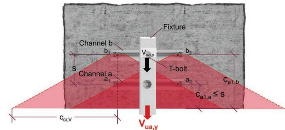
Figure 9.2.13.5 — Parallel Channels-Shear Casel-Plan view.
