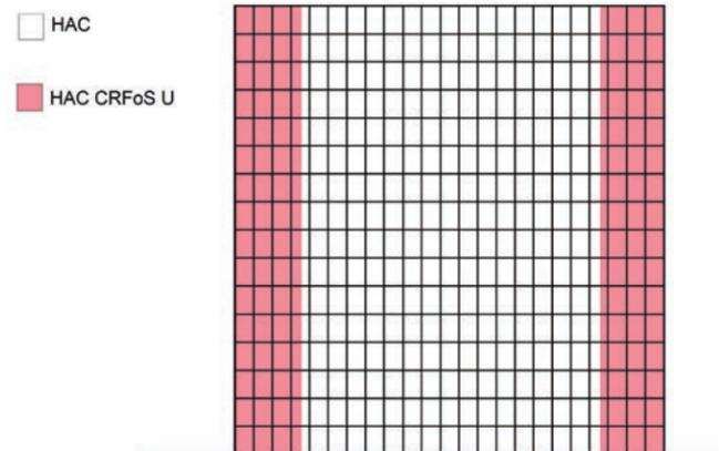
Figure 12.4.1.2 Optimum anchor channel layout
