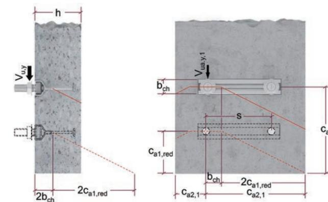
Figure 7.4.2.8 — Example of an anchor channel influenced by two corners and member thickness (in this example  $c_{a2,2}$  is decisive for the determination of  $c_{a1,red}$ )
