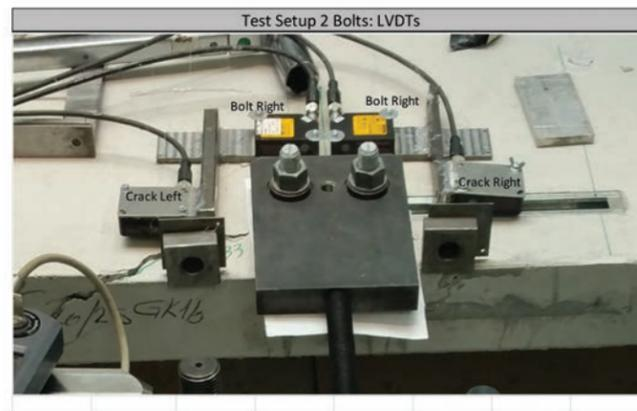
Figure 9.6.2.14 — Test Setup 2 Bolts: LVDTs.
