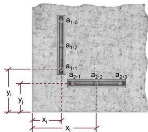
Figure 9.2.10.7 – definition of the relative distance of the anchors in an anchor channels group.
