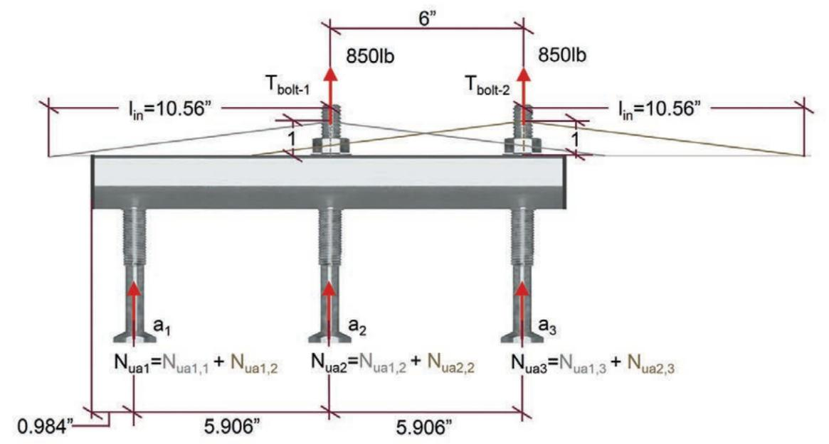
Figure 14.1.11 — Design example – Anchor Tension Forces
