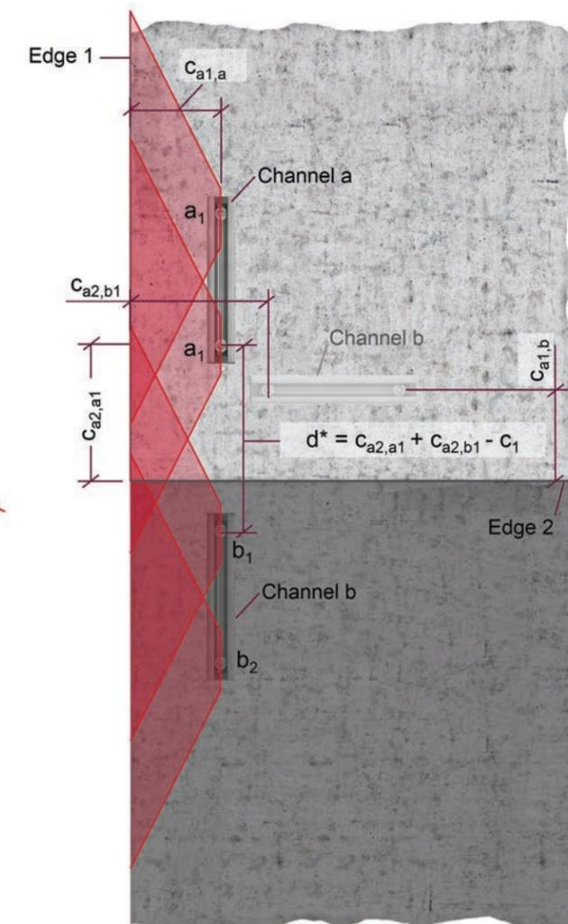
Figure 9.2.10.11d — Unfolding of the corner.
