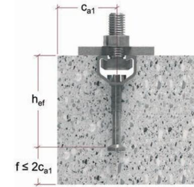
Figure 7.3.2.19 — Anchor channel at the edge of thin concrete member
