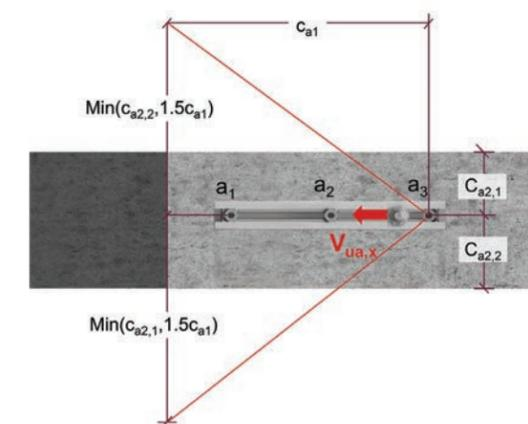
Figure 9.2.2.7 — Obtuse corner — Longitudinal shear — Plan view.
