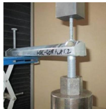
Figure 7.3.1.1 — Tension test for testing anchor channels in a universal testing machine.
