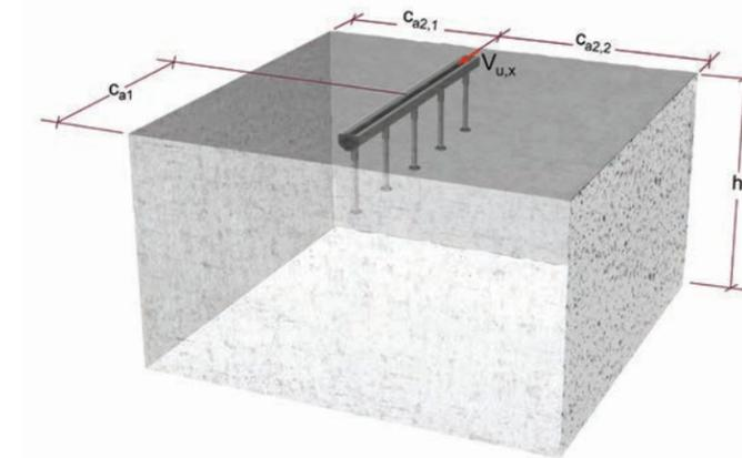
Case I: Concrete edge failure governs,  $\Psi_{parallel}=1.0$
