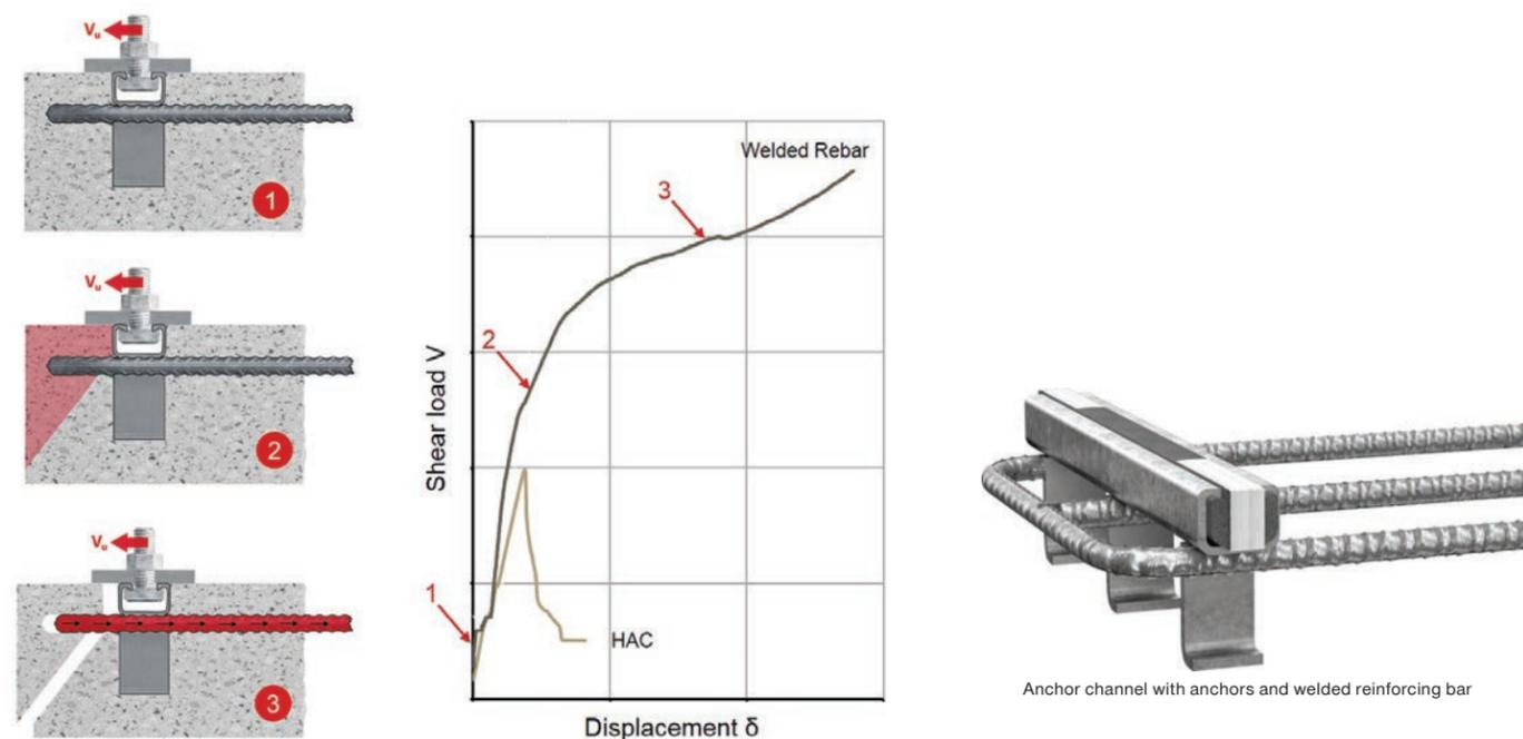
Figure 9.6.1.4 — Welded rebar channel — Behavior of anchor channels with reinforcing bars loaded in shear (left). Shear load vs displacement curve (right).
