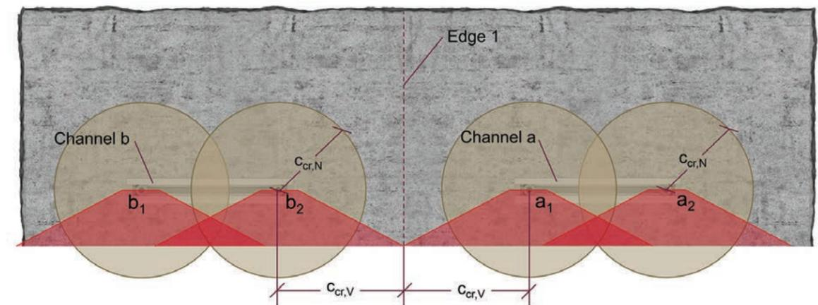
Figure 9.2.8.1 — TOS and BOS with pair of anchor channel adjacent to each other — Tension and perpendicular capacity doesn't get reduced.
