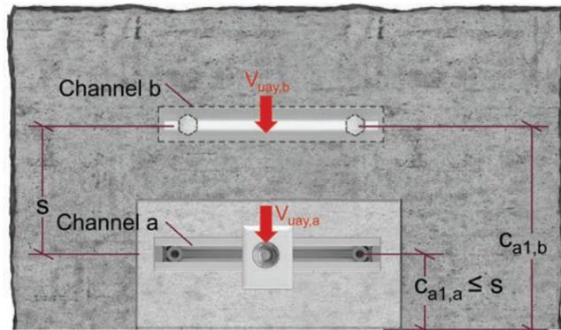
Figure 9.2.14.1 — Parallel Channels Top and Bottom: BOS away from TOS - Plan View.
