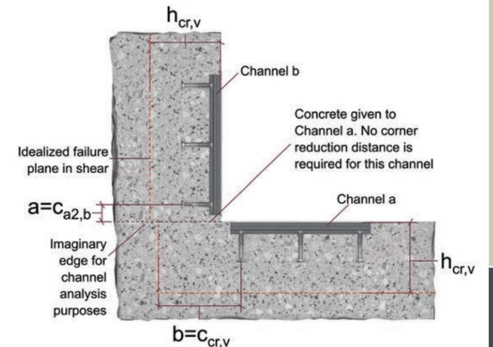
Figure 9.2.4.2 — Acute angle interior FoS corner with anchor channels on both sides — Perpendicular shear.
