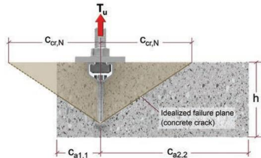
Figure 7.3.2.11 - Idealize failure plane in concrete due to tension forces.
