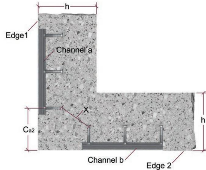
Figure 9.2.6.1 — Example of design of FOS outside corner.
