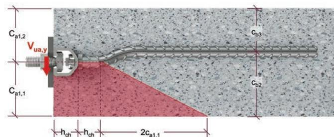
Figure 9.3.3.7 — HAC CRFOS U — Anchor channels on both sides — Obtuse angle Corner — Section View.
