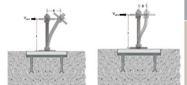
Figure 7.4.3.2— Channel bolt resisting shear forces with stand off.
