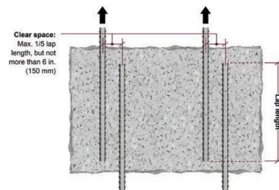
Figure 8.6.1.5 — Non-contact lap splice.
