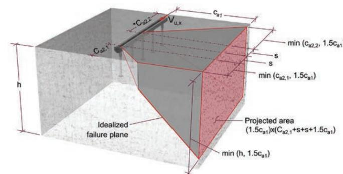
Figure 7.4.4.4 – Projected area due to an anchor channel loaded in shear acting parallel to the long channel axis. Verification of side concrete edge breakout.
