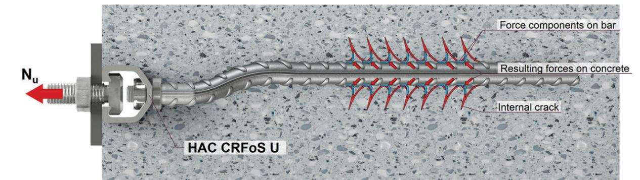
Figure 9.3.1.2 — Cast-in anchor channel with reinforcing bar anchors (HAC CRFoS U) loaded in tension.
