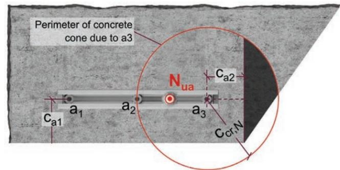
Figure 9.2.7.3 — Obtuse angle corner — TOS or BOS single channel at certain distance — Tension.
