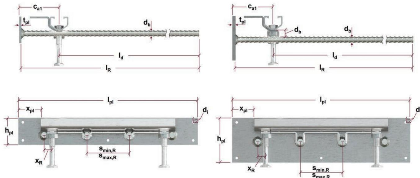
**Figure 2.2.16.13 — HAC-T S EDGE dimensions, section and elevation view.**
