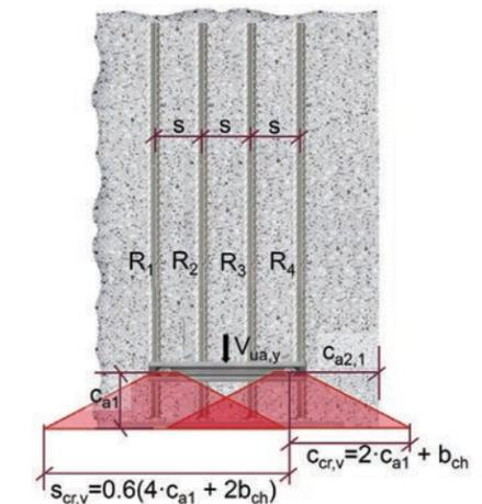
Figure 9.6.4.2 — TOS or BOS HAC EDGE single channel — Shear along perpendicular to axis y+.
