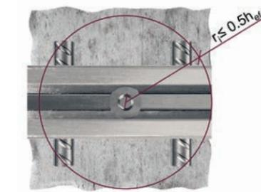
Figure 7.3.2.17 — Arrangement of anchor reinforcement for anchor channels loaded in tension, plan view.
