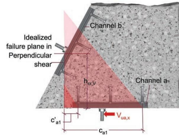
Figure 9.2.3.14 – Acute FoS corner with anchor channels on both sides – Effect of longitudinal, perpendicular shear and tension.
