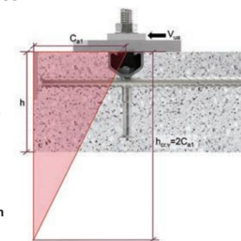
Figure 9.6.2.6 – Modification of height  $\Psi_{h,v}$
