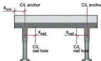
Figure 2.2.1.3 b – HAC end and nail hole distance.
