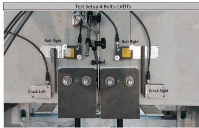
Figure 9.6.2.13 — Test Setup 4 Bolts: LVDTs.
