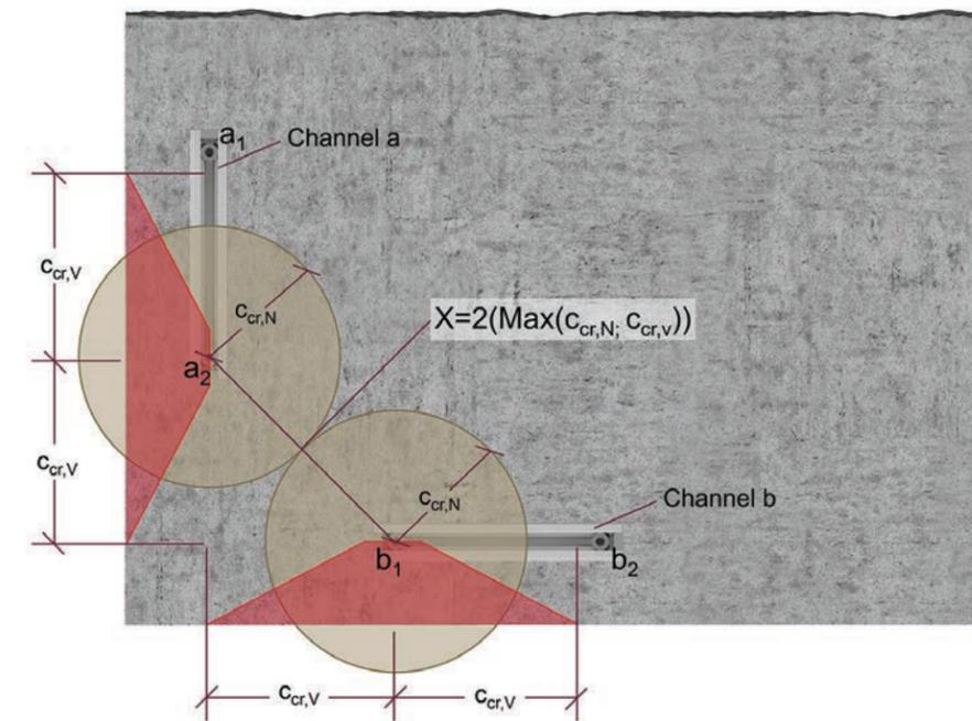
Figure 9.2.9.1 — TOS and BOS outside corner — Tension and perpendicular shear concrete cones does not intersect.
