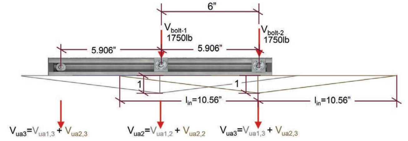
Figure 14.1.15 – Design example – Anchor Shear forces
