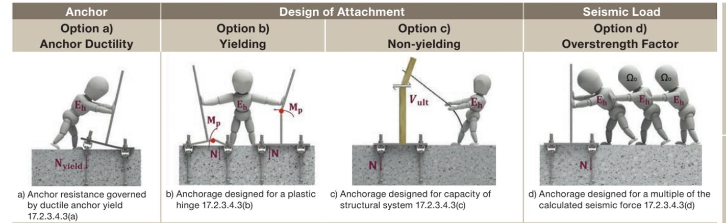
Figure 7.6.2.1— Seismic provisions for tension; ACI 318-14 Section 17.2.3.4.3.
