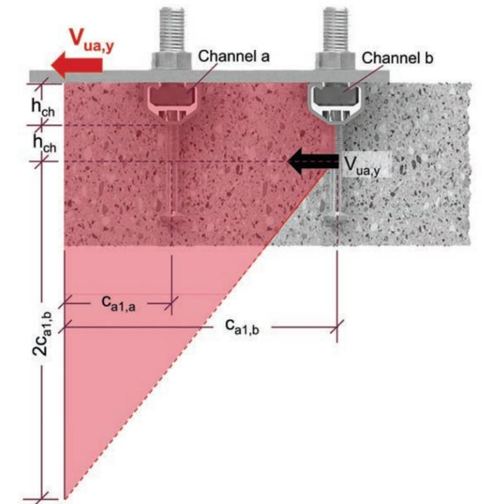
Figure 9.2.13.6 — Parallel Channels-Shear Case II-Section view.
