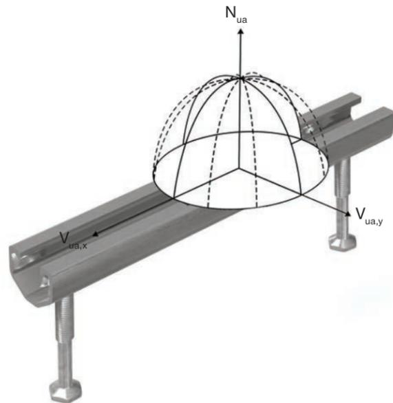
Figure 7.2.3.1 — Anchor channel loaded in three directions.
