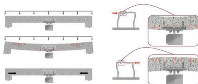
The crack opens and closes with the changing of live load and rebar restraint, which is less severe compared to seismic conditions.
