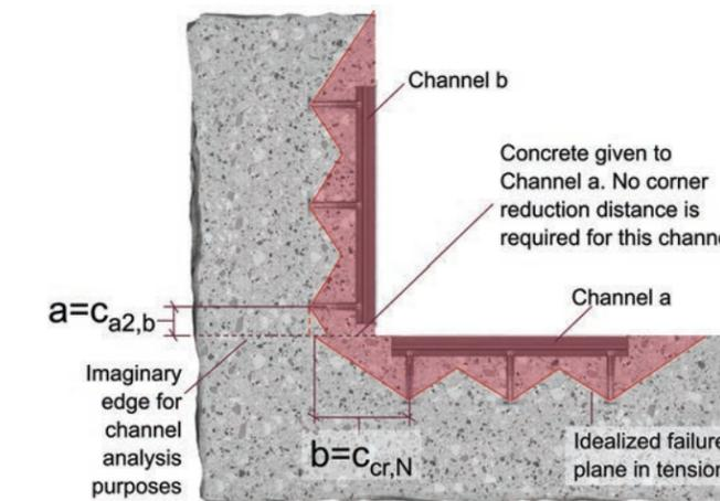
Figure 9.2.4.1 — 90° interior FoS corner with anchor channels on both sides.
