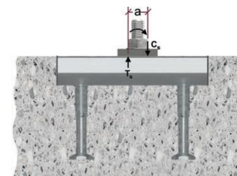
Figure 7.4.3.1 — Definition of lever arm.
