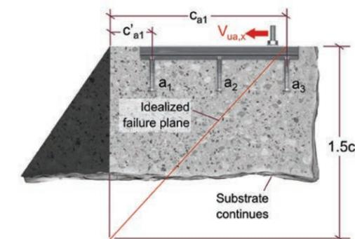
Figure 9.2.2.6 — Obtuse corner — Longitudinal shear — Section view.
