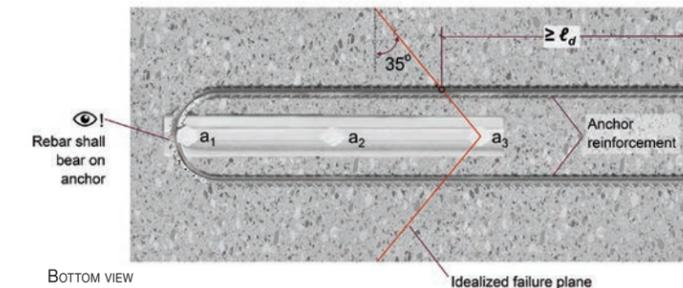
Figure 7.4.4.5 – Anchor reinforcement to preclude concrete breakout in shear acting along the longitudinal axis of the anchor channel
