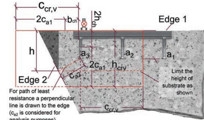
Figure 9.2.2.9 — Acute corner — Perpendicular shear — Section view.
