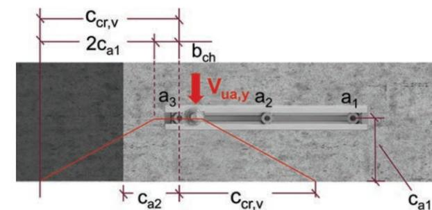
Figure 9.2.2.5 — Obtuse corner — perpendicular shear — Plan view.
