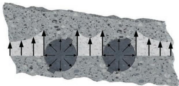
Figure 8.6.1.3 - Radial forces on concrete and splitting stresses shown on section through the splice.
