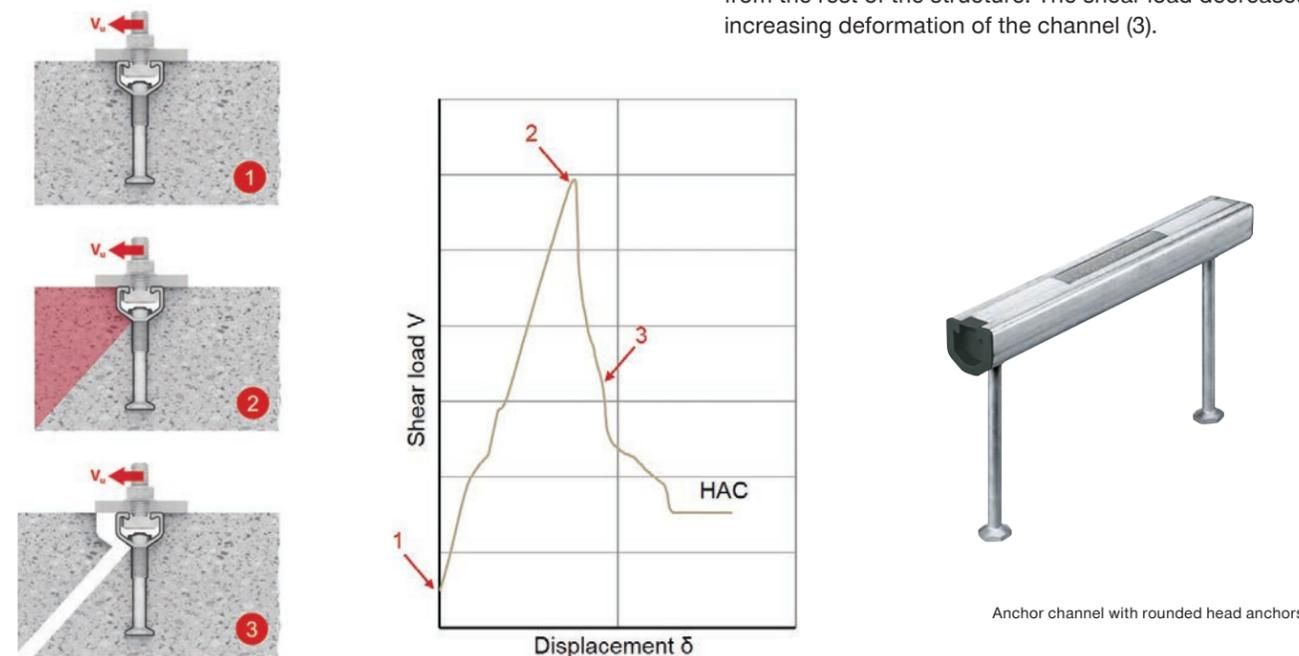
Figure 9.6.1.3 — HAC — Headed Studs — Behavior of anchor channels loaded in shear (left). Shear load vs displacement curve (right).
