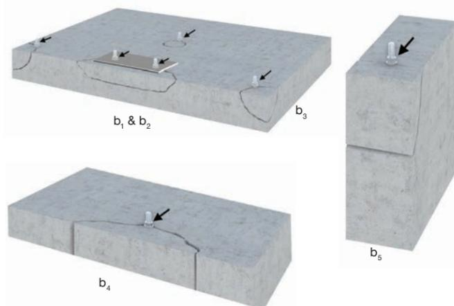
Figure 7.4.2.2 — Failure of concrete breakout in shear b<sub>1</sub>, b<sub>2</sub> and b<sub>3</sub>) close to an edge, close to an edge and corner, away from the edge b<sub>4</sub> close to an edge, b<sub>5</sub> close to an edge and two corners in a deep member.
