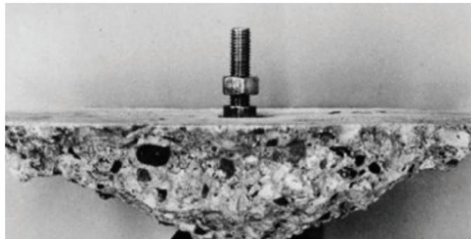
Figure 7.3.2.5 — Concrete cone in tension. (Picture from Anchorage in Concrete Construction, R. Eligehausen).
