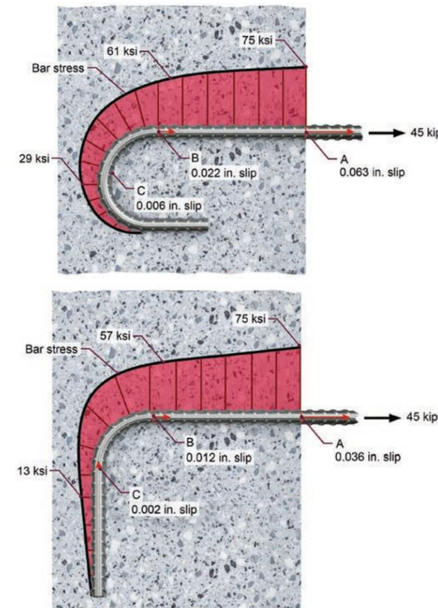
Figure 8.5.1.2 — Stresses in 90 and 180 degree hooks. Source: Wight, James & MacGregor, James. Reinforced Concrete Mechanics & Design, 2012.
