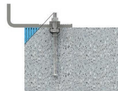
Figure 7.2.7.1 — Distribution of forces predicted by elastic theory in a t-bolt group subjected to tension force and bending moment.
