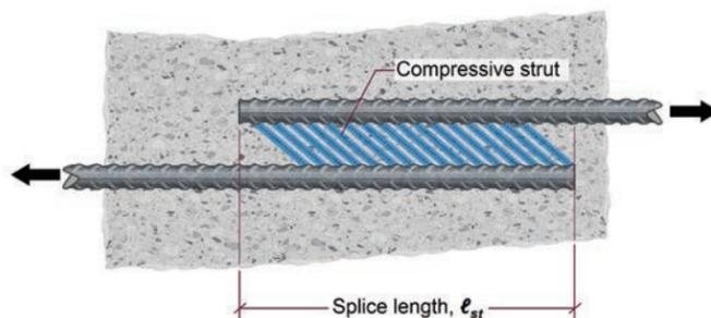
Figure 8.6.1.2 — Compressive struts at splice.
