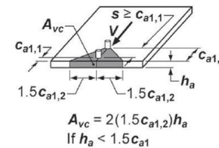
Figure 9.2.13.4 — Fig. R17.5.2.1b — Calculation of  $A_{vc}$  for single anchors and groups of anchors per ACI 318-14..
