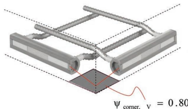
Figure 9.3.3.3 — HAC CRFOS U — Anchor channels on both sides — 90 degree angle Corner — Reduction factor.
