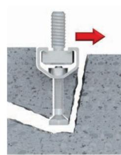
Failure load associated with pry-out; The load-bearing mechanism of a single headed stud anchorage subjected to a shear load is illustrated schematically in Fig 7.4.2.10. The applied shear load gives rise to bearing stresses in the concrete. With increasing load the surface concrete is crushed or spalled, shifting the centroid of resistance  $V_b$  to a location deeper in the concrete.
