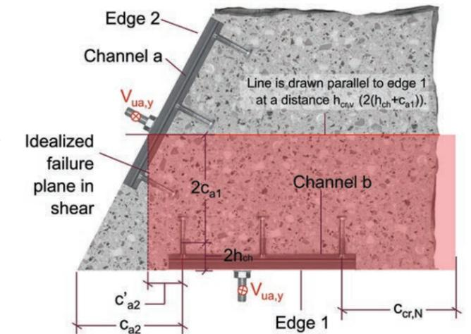
Figure 9.2.3.12 – Acute angle FoS corner with anchor channels on both sides – Perpendicular shear analysis- Section view.
