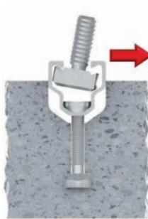
The nominal strength of one anchor, V<sub>sa,y</sub>, and anchor and channel connection V<sub>sc,y</sub> to take up shear loads perpendicular to the channel must be taken from Table 8-5 for HAC and HAC-T with Hilti channel bolts (HBC-B, HBC-C, HBC-T and HBC-C-N).
