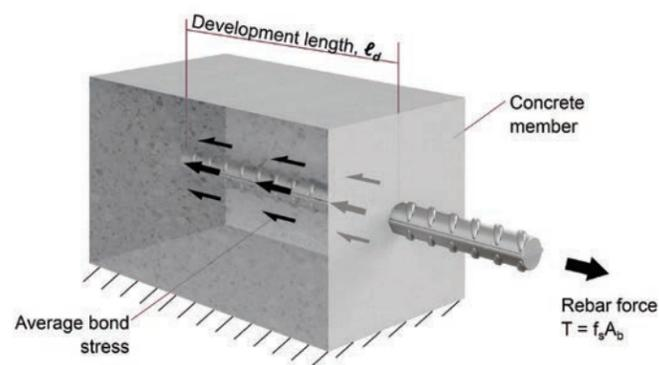
Figure 8.1.1.1 — Bond stresses on a reinforcing bar.
