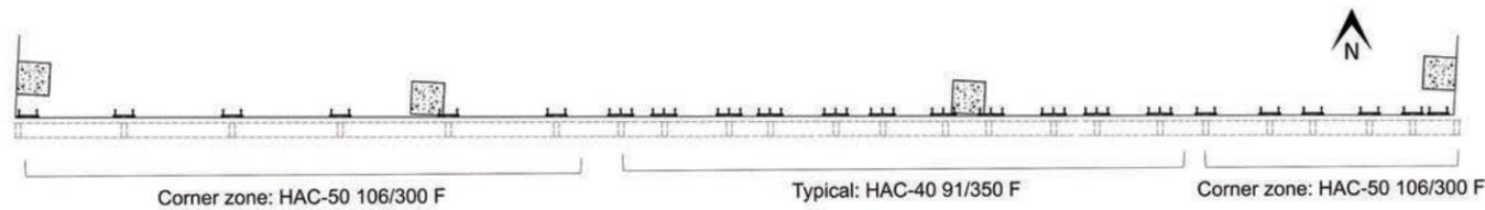
Figure 11.2.3.1 Embed layout, plan view
