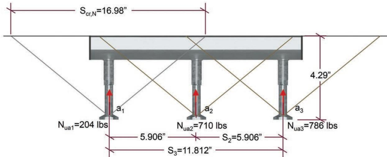
Figure 14.1.19 — Design example – spacing reduction factor -  $S_{cr,N}$
