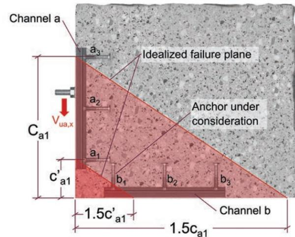
Figure 9.2.3.8 – 90° FoS corner with anchor channels on both sides – Effect of longitudinal, perpendicular shear and tension.
