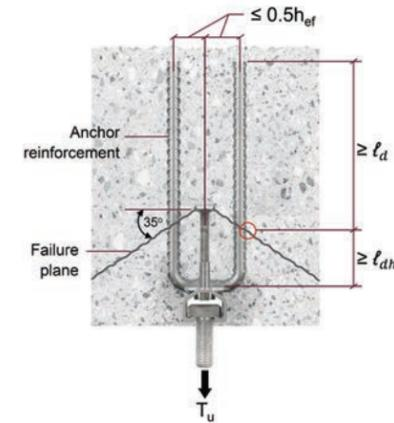
Figure 7.3.2.15 — Arrangement of anchor reinforcement for anchor channels loaded by tension load in a narrow member.
