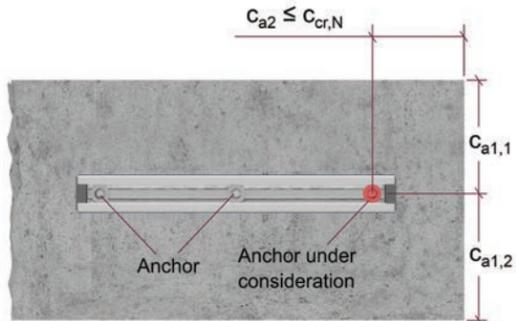
Figure 7.3.2.9 — Anchor channel with influence of two edges and one corner.
