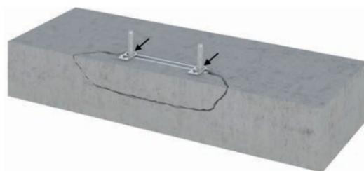
Figure 7.4.2.1 — Concrete edge failure due to an anchor channel loaded in shear. Spacing of anchors equal to 5 times the edge distance
