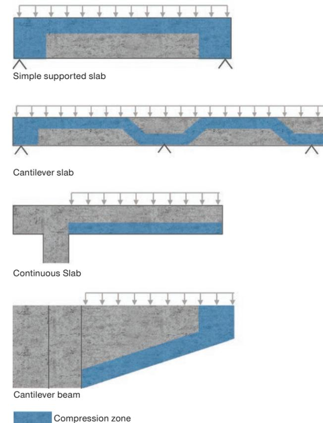
Figure 11.5.4.1 — Compression zones in different concrete structures
