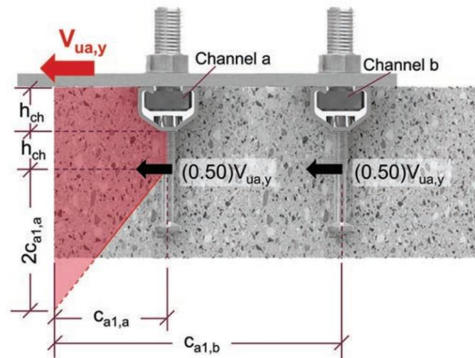
FFigure 9.2.13.3 — Parallel Channels — Shear Casel-Section view.
