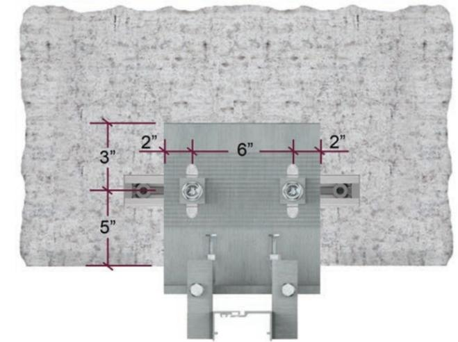
Figure 14.1.3 — Design example - Bracket Plan View
