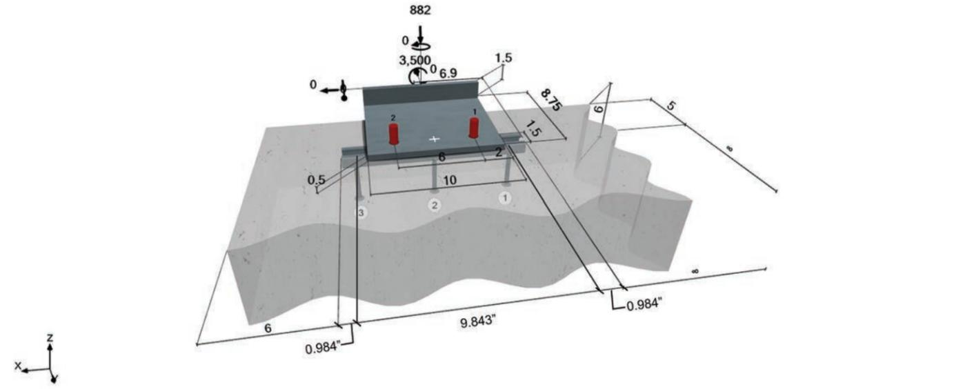
Figure 14.1.9 — Design example – Profis anchor channel - 3D Back View
