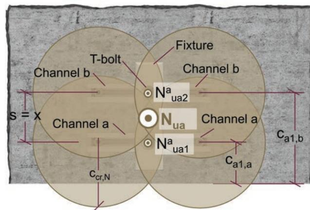
Figure 9.2.13.9 – Tension – Equal tension force-Plan view.
