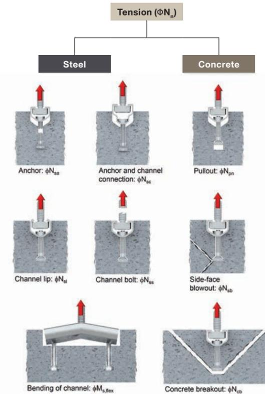
Figure 7.3.1 — Possible tensile failure modes of an anchor channel.
