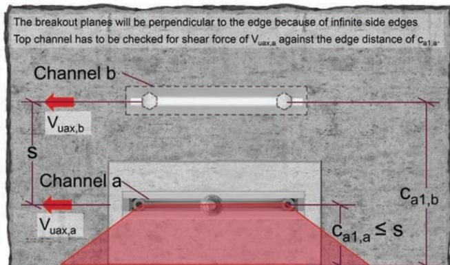
Figure 9.2.14.10-a — Longitudinal Shear — Plan view-Top anchor channel.
