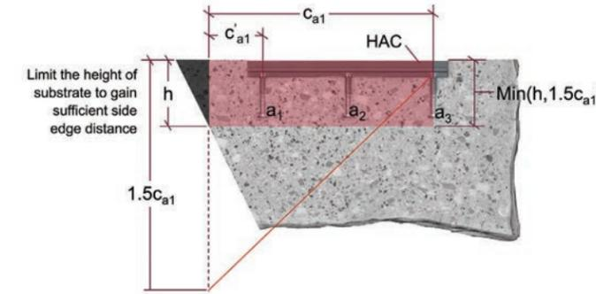
Figure 9.2.2.11 — Acute corner — Longitudinal shear — Section view.
