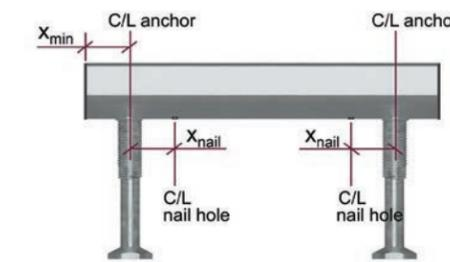
Figure 2.2.13.5 a — HAC end and nail hole distance.
