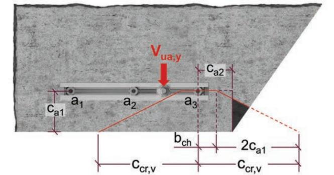
Figure 9.2.7.2 — Obtuse angle corner — TOS or BOS single channel at certain distance — Perpendicular Shear.
