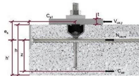
Figure 9.6.2.10 — Anchor reinforcement to resist shear loads.
