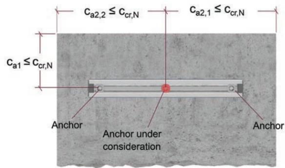
Figure 7.3.2.8 — Anchor channel with influence of one edge and two corners.
