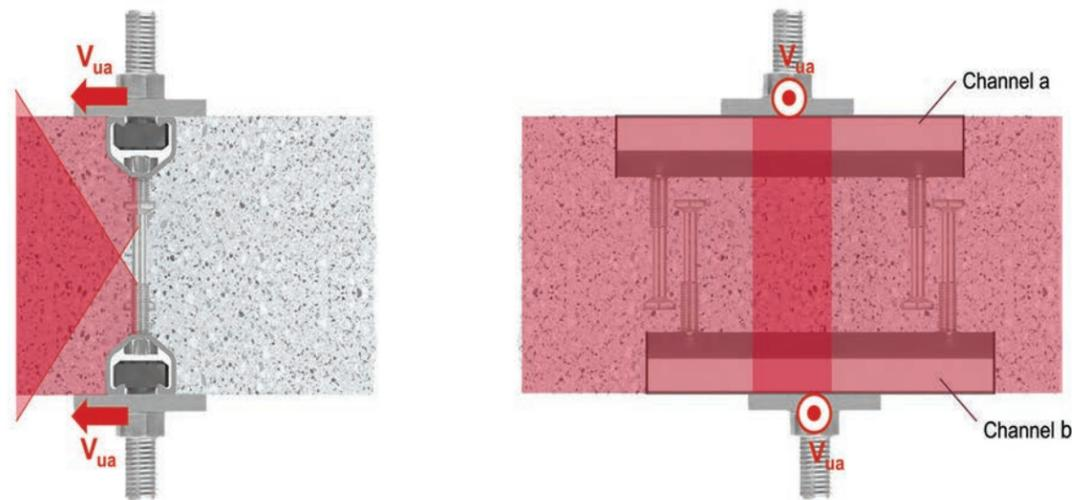
Figure 9.2.14.14 — Intersecting Top and Bottom Channel; shear loading
