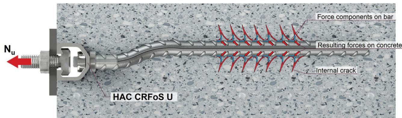
State-of-art design model based on ICC ESR-3520 and principles of AC232 and ACI 318. 19 out of 20 possible failure modes are calculated in accordance with AC232.
