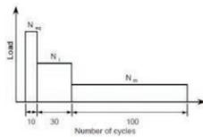
Figure 7.6.4.1 — Required load history for simulated seismic tension test
