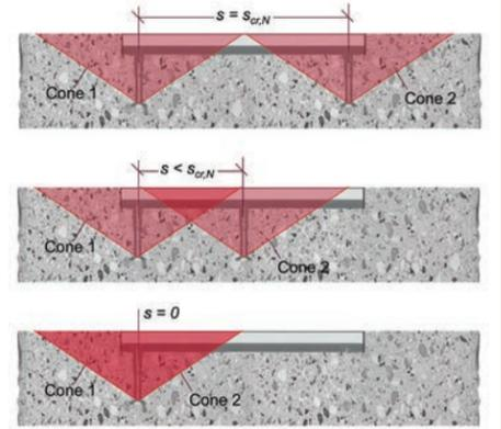
Figure 9.2.10.3 —  $\psi_{s,N}$  for two anchors symmetrically loaded.
