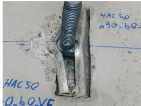
Figure 7.4.1.1 — Steel failure in shear of anchor channel lip.
