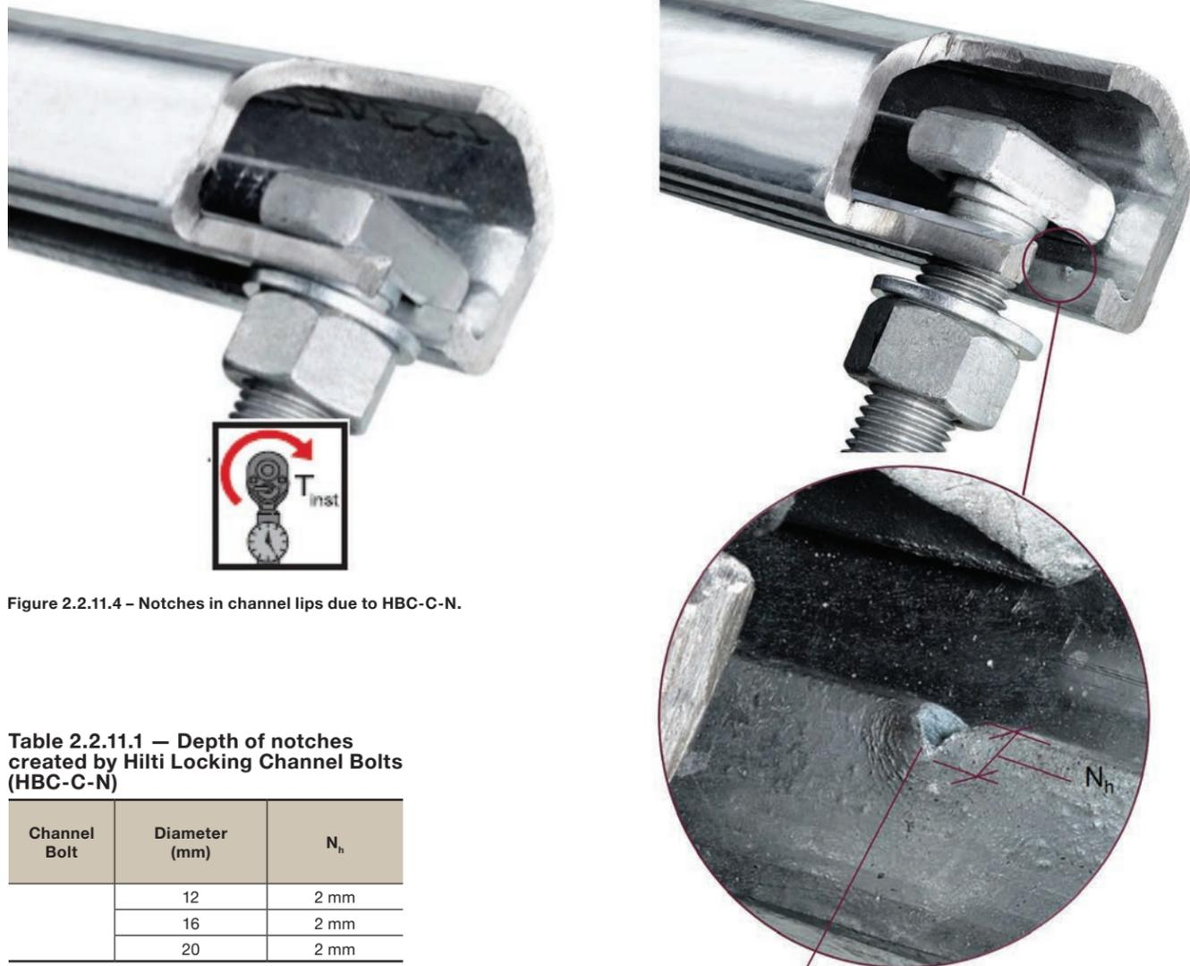
Figure 2.2.11.4 – Notches in channel lips due to HBC-C-N.
