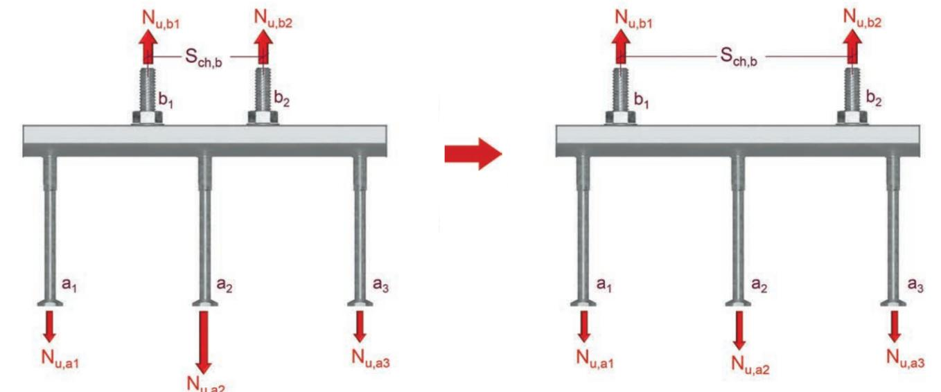
Figure 11.3.1.1 optimization of load distribution from t-bolts to anchors
