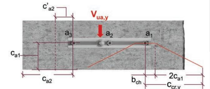
Figure 9.2.3.11 – Acute angle FoS corner with anchor channels on both sides – Perpendicular shear analysis – Plan view.
