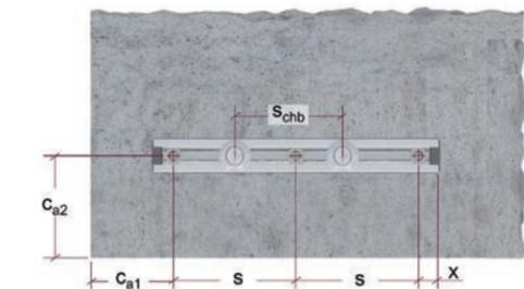
Figure 7.2.2.5 — Plan view of an anchor channel system in a concrete member.
