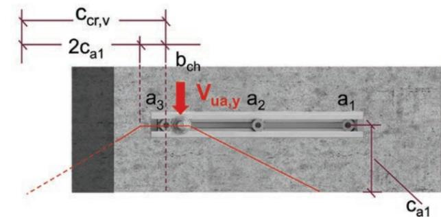
Figure 9.2.2.10 — Acute corner — Perpendicular shear — Plan view.
