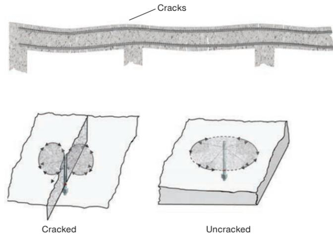
Figure 7.3.2.14 — Cracked and uncracked concrete.
