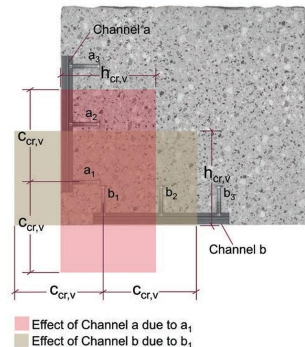
Figure 9.2.3.4 – 90° FoS corner with anchor channels on both sides – Determination of b.
