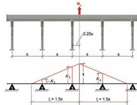
Figure 7.2.8.1 — Example for the calculation of anchor forces in accordance with the triangular load distribution method for an anchor channel with five anchors. The influence length is assumed as  $l_{in} = 1.5s$ .
