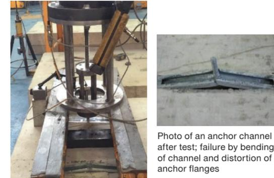
Figure 7.3.1.7 — Flexural test on anchor channels.
