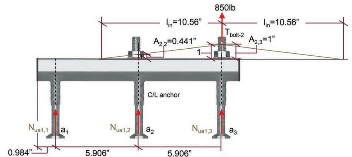
Figure 14.1.13 — Design example – effect of t-bolt 2 on anchors
