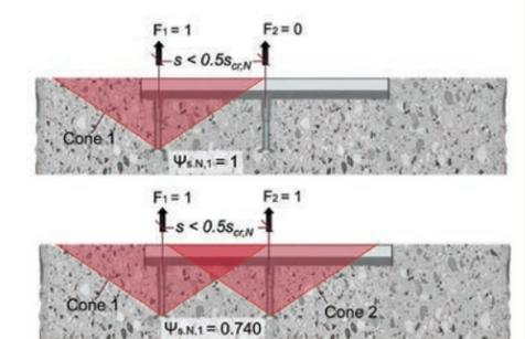
Figure 9.2.10.5 — Influence on  $\psi_{s,N,1}$  (of the anchor 1) of the relative load on the anchors.
