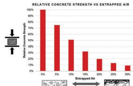
Figure 11.5.6.2 — Loss of Concrete Compressive Strength Through Increase in Entrapped Air (2).
