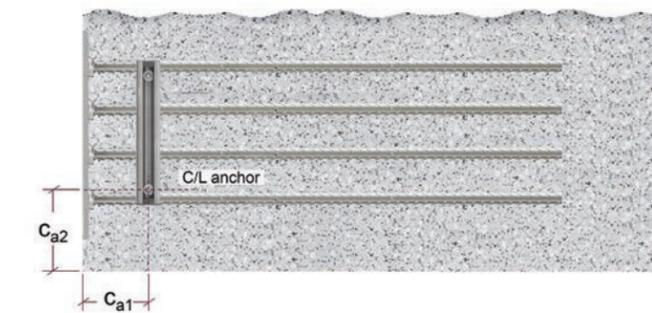
Corner and edge distances are measured to the center of the anchor.
