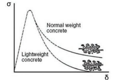
Figure 7.3.2.1 — Influence of crack path on the stress-deformation behavior of concrete. (Picture from Anchorage in Concrete Construction, R. Elgehausen).
