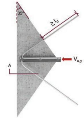
Figure 7.4.4.6 – Anchor reinforcement to resist shear loads acting along the longitudinal axis of the anchor channel.
