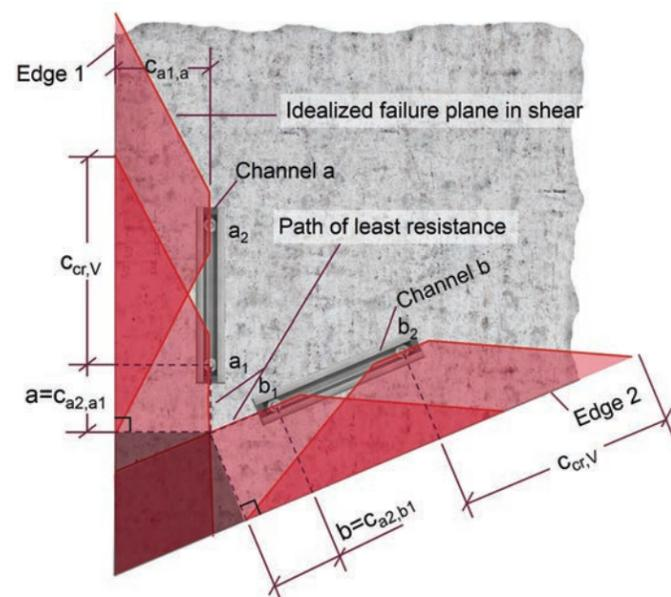
Figure 9.2.10.17-b — Simplified Method — Acute Corner — Perpendicular Shear.
