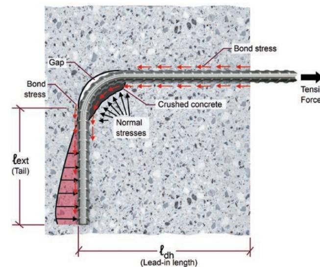
Figure 8.5.1.1 — Stresses in standard 90 degree hook. Source: Wight, James & MacGregor, James. Reinforced Concrete Mechanics & Design, 2012.
