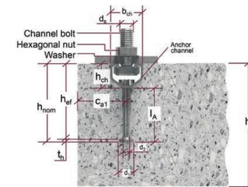
Figure 7.2.2.6 — Section view of an anchor channel system in a concrete member.
