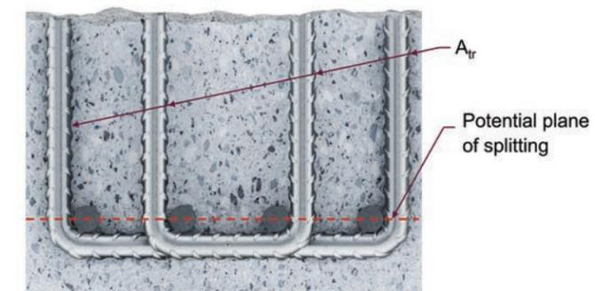
Figure 8.1.1.4 — Potential plane of splitting due to closely spaced reinforcing bars.
