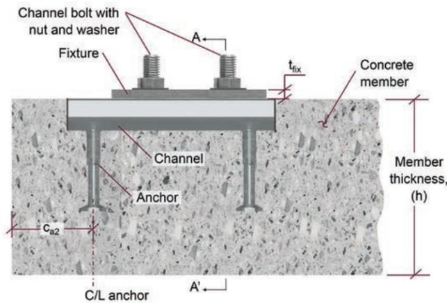
Elevation view of an anchor channel system.
