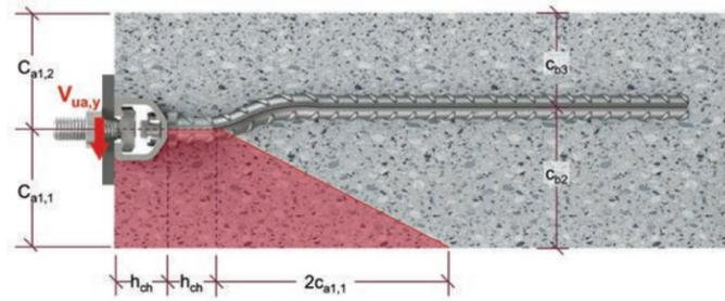
Figure 9.3.3.2 — HAC CRFOS U — Anchor channels on both sides — 90 degree angle Corner — Section View.
