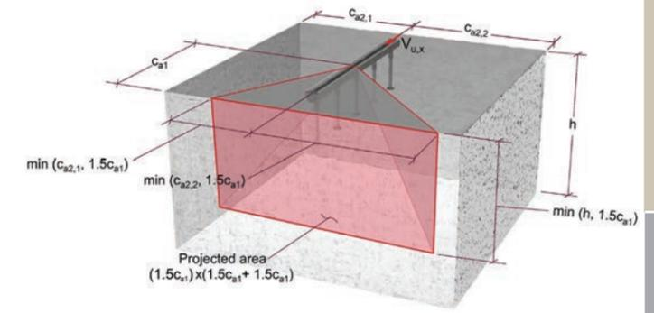
Figure 7.4.4.2 — Projected area due to an anchor channel loaded in shear acting parallel to the long channel axis. Full shear loading acting on the 3rd anchor away from the edge.
