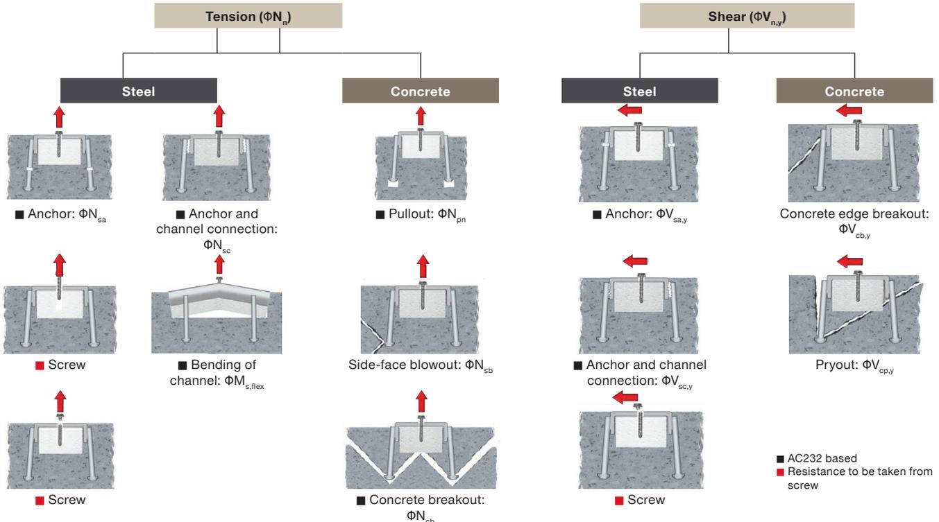
Verification of superposition of tension and shear loads must be verified
