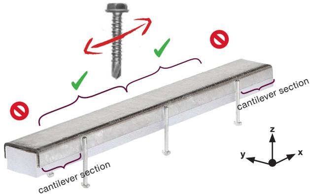
Figure 6 — Allowed screws position on HAC-TU along the longitudinal x) axis
