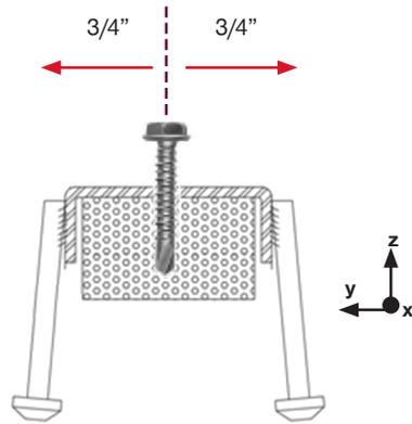
Figure 7 — Allowed screws position on HAC-TU along the perpendicular (y) axis
