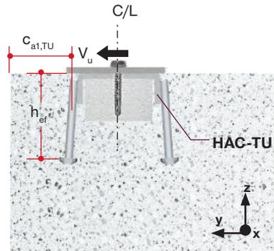
Figure 4b — Edge distance ( $C_{a1}$ ) for analysis purposes of an inverted cast-in channel such as HAC-TU, for analysis purposes
