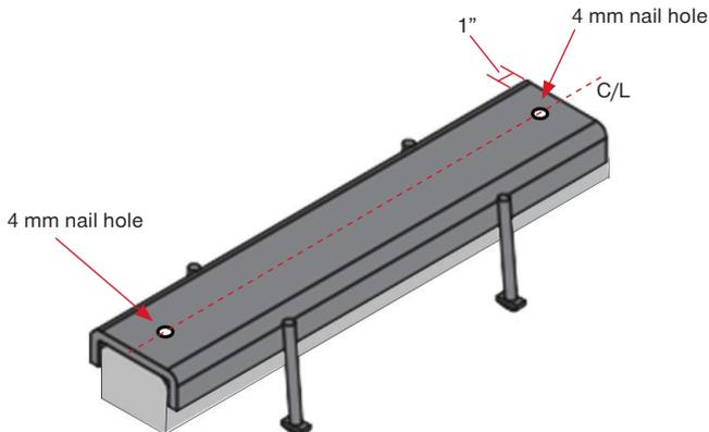
Figure 10 – HAC-TU cut in shorter sections and nail holes added
