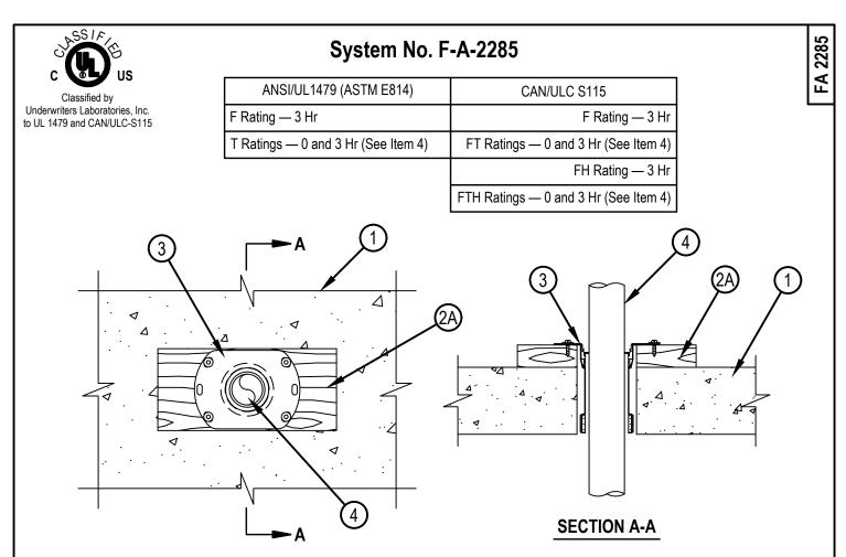
System tested with a pressure differential of 2.5 Pa between the exposed and the unexposed surfaces with the higher pressure on the exposed side.
