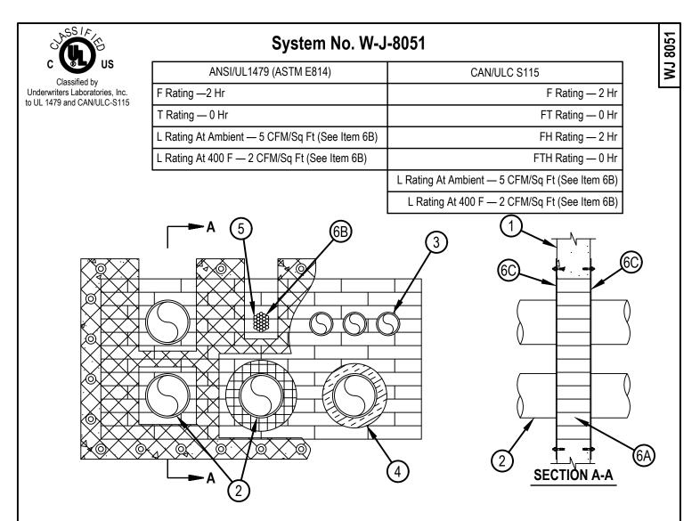
System tested with a pressure differential of 2.5 Pa between the exposed and the unexposed surfaces with the higher pressure on the exposed side.
