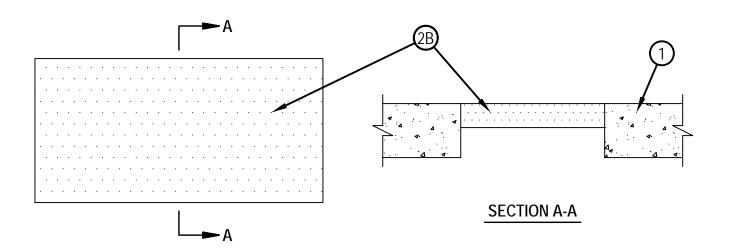
1. Floor or Wall Assembly -- Min 4-1/2 in. thick reinforced lightweight or normal weight (100-150 pcf) concrete. Wall may also be constructed of any UL Classified Concrete Blocks\*. Max area of opening is 288 sq in. with max dimension of 24 in.
