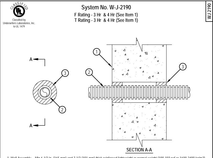
1. Wall Assembly -- Min 6-1/2 in. (165 mm) and 7-1/2 (191 mm) thick reinforced lightweight or normal weight (100-150 pcf or 1600-2400 kg/m3) concrete for 3 and 4 hr fire rated wall assemblies, respectively. Wall may also be constructed of any UL Classified Concrete Blocks<sup>\*</sup>. Max diam of opening is 3-1/2 in. (89 mm).
