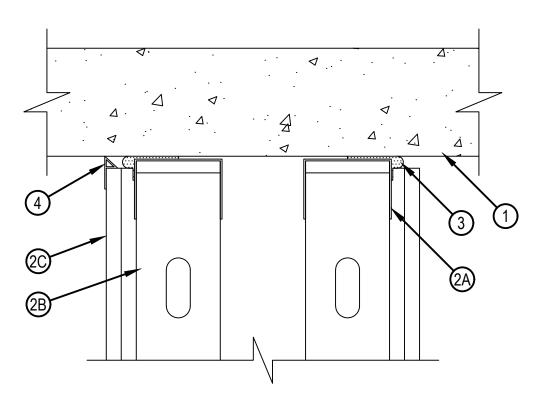
1. Floor Assembly — Min 4-1/2 in. (114 mm) thick reinforced lightweight or normal weight (100-150 pcf or 1600-2400 kg/m3) structural concrete. Floor may also be constructed of any 6 in. (152 mm) thick UL Classified hollow-core Precast Concrete Units\*.
