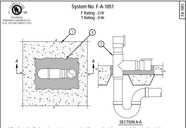
1. Floor Assembly -- The fire rated unprotected concrete and steel floor assembly shall be constructed of the materials and in the manner specified in the individual D900 Series designs in the UL Fire Resistance Directory and as summarized below:
