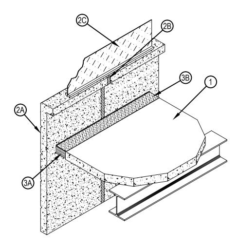
1. Floor Assembly — Min 5 in. (127 mm) thick steel-reinforced lightweight or normal weight (100-150 pcf or 1600-2400 kg/m3) structural concrete. Floor assembly to be supported at perimeter edges by spandrel beams having a Restrained or Unrestrained Beam Rating of 3 hr.
