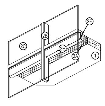
1. CONCRETE FLOOR ASSEMBLY: 2 hour rated concrete floor assembly made from either lightweight or normal weight concrete with a density of 100 to 150 pcf, having a min. thickness of 6 in. at the joint face. When a longitudinal recess (blockout) is required to contain an architectural joint system, increase concrete floor assembly thickness to maintain a min. thickness of 6 in. and accommodate depth of blockout formed in the concrete: blockout width unrestricted.
