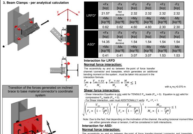
The eccentricity ey and ez between the point of force transfer channel / connector and baseplate, which generates an additional bending moment on the system , must be taken into account in the interaction formula.
