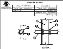
(all Assembly — The 1 or 2 hr fire-rated gypsum board/stud wall assembly shall be constructed of the materials and in the manner specified in e individual U300, U400, V400 or W400 Series Wall and Partition Designs in the UL Fire Resistance Directory and shall include the following
