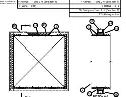
Wall Assembly — The 1 or 2 hr fire-rated gypsum board/stud wall assembly shall be constructed of the materials and in the manner specified he individual U300, U400, V400 or W400 Series Wall and Partition Designs in the UL Fire Resistance Directory and shall include the followin
