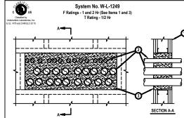
Wall Assembly The 1 or 2 hr fire-rated gopsom boardistud wall assembly shall be constructed of the materials and in the manner described in the individual UAO Series Wall or Partition Design in the UL Fire Resistance Directory and shall include the following construction features.
