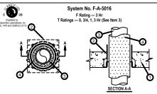
Floor Assembly — Min 4-1/2 in. (114 mm) thick reinforced lightweight or normal veight (100-150 pcf or
